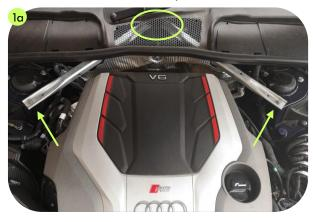
Step 2 - Removal of OEM Strut Brace:
