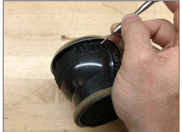
**2a** Using a small screwdriver release the tab on the bottom of the vent (6 O'clock position)
