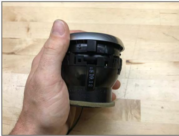
**10** Reinstall trim ring onto vent housing
