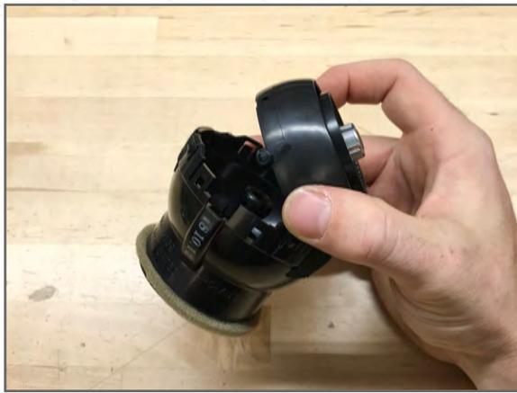
**6** Remove slat assembly from housing
