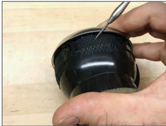
**2b** Release three remaining tabs under felt at 3, 9, and 12 O'clock positions
