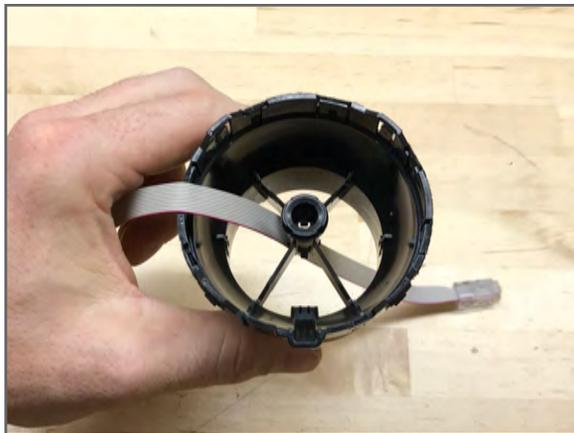
**8** Feed display cable through housing as shown
