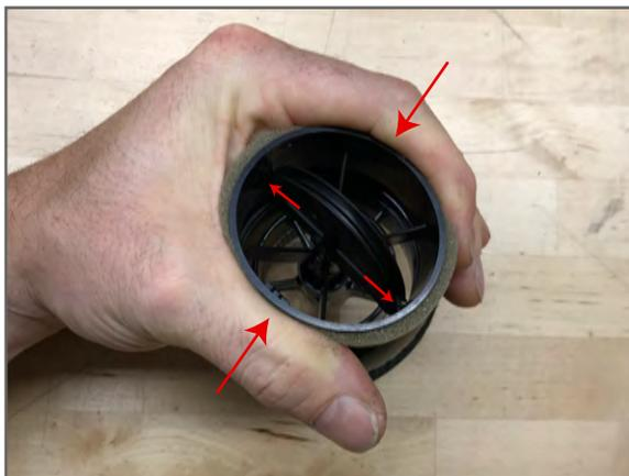
**4** Squeeze vent into oval shape to release flap pins
