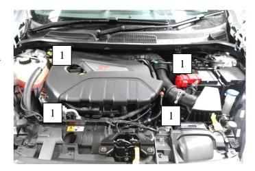
2. Locate the MAP sensor. When facing the vehicle, the MAP sensor is located on the left hand side of the engine on the intake plenum.
