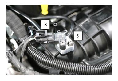
9. Your boost reference adapter is now installed. Reinstall engine cover.
