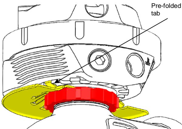
Tighten the collar using a torque wrench on the 3/8" square drive provided in the collar tool perpendicular to the length of the tool to **25N.m (18ft/lbs)**. Fold down a tab onto the slave collar to prevent the collar from coming loose during use.
