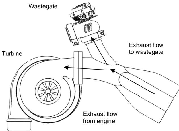
Figure 4 - Best flow - Symmetric mounting
