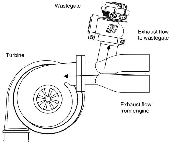
Figure 7 - **Not Recommended** - Less than 90 Degree Mounting
