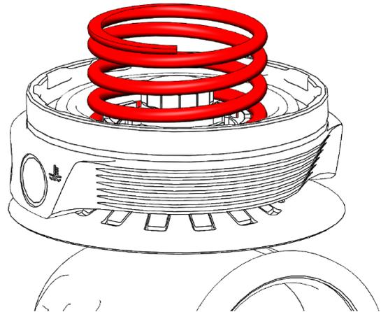
Configure wastegate with preferred spring combination of inner, middle and outer springs
