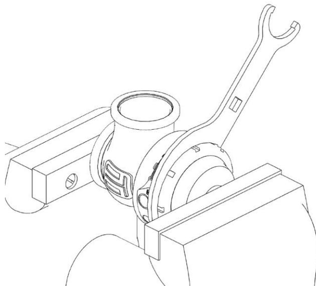
Reinstall fittings to the cap of the wastegate using fresh Loctite 567 thread sealant.
