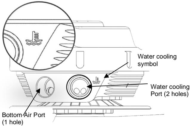
Fit water cooling port fittings Prior to mounting the wastegate, install 1/8" NPT fittings into the water ports, apply thread lubricant and screw in clockwise until finger tight, then tighten further 1-2 turns for seal. Choose feed and drain source for the water and connect to the wastegate. Turbosmart recommends -4SAE fittings and hose compatible with coolant.
