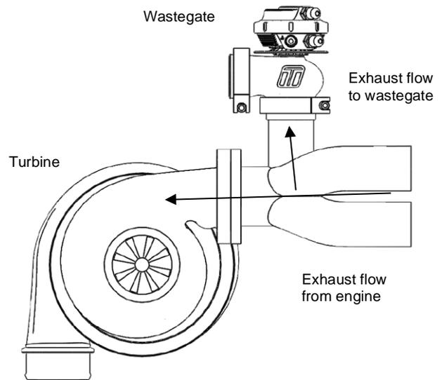
Figure 6 - 90 Degree mounting
