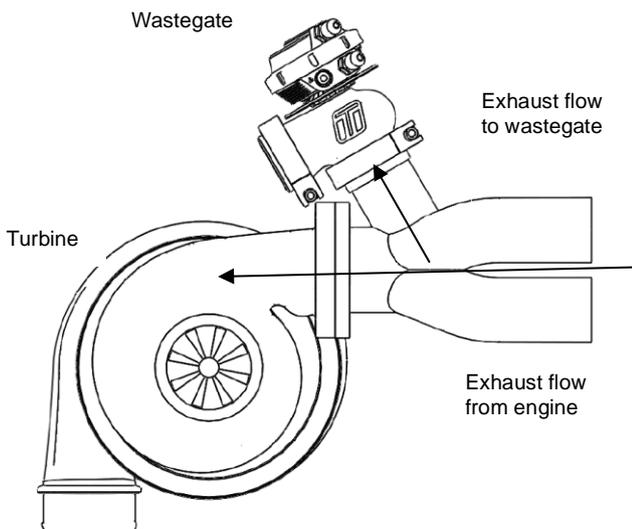
Figure 5 - Good Flow - Angle mounting
