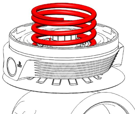
Configure wastegate with preferred spring combination of inner, middle and outer springs
