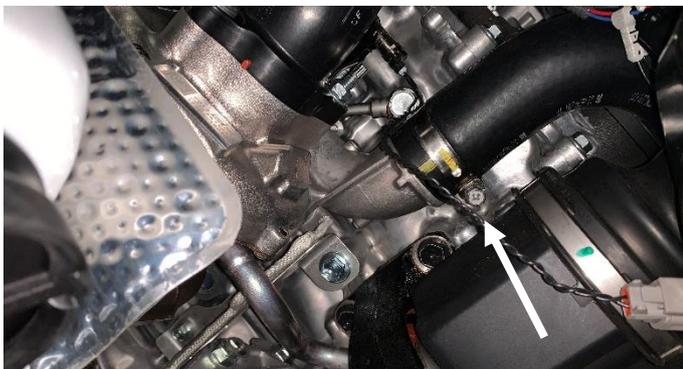
Pictured above is the hose clamp that will need to be removed. It is located on the turbo snout.
