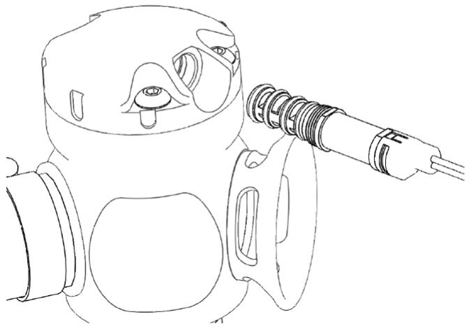
Tighten the new solenoid into the EM series BOV ensuring the wrench is on the metallic portion of the solenoid.
