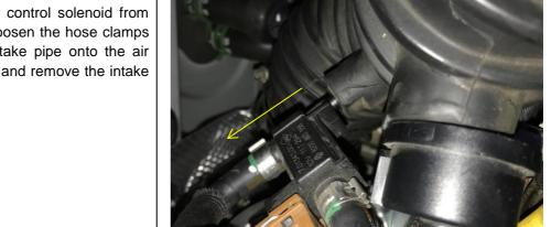
5. Locate the vacuum hose on the OEM recirculation valve and trace it to the tee piece, undo the hose clamp by
