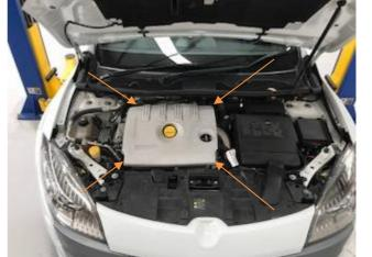
2. Disconnect the PCV return from the inlet hose by pressing the yellow tab firmly and lifting. The larger hose slides off the tee piece. Rotate the hose out of the way, or remove it completely if required.
