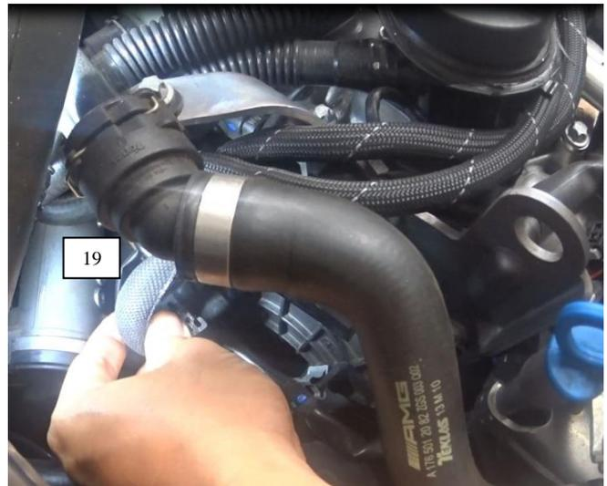
20. Remove the factory hose off the in the intake manifold. The manifold port is shown below. Note: this is the port after factory hose has been removed.
