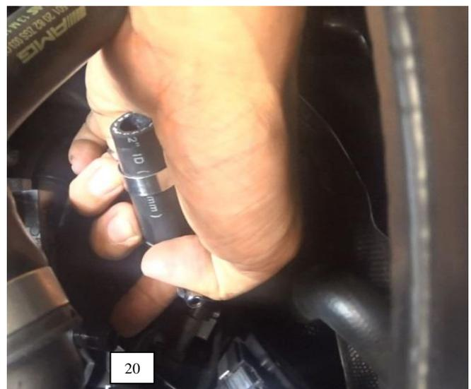
21. Install the OEM hose onto the smaller barb side of the boost reference adapter. Use the OEM spring clamp to secure the hose onto the boost reference adapter.
