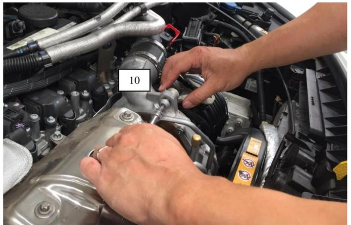
11. Loosen hose clamp and remove the intake muffler.
