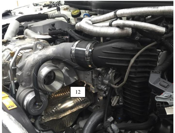
13. Remove the three bolts securing the BOV blanking plate onto the turbocharger compressor cover. Remove BOV blanking plate once all three bolts have been removed.
