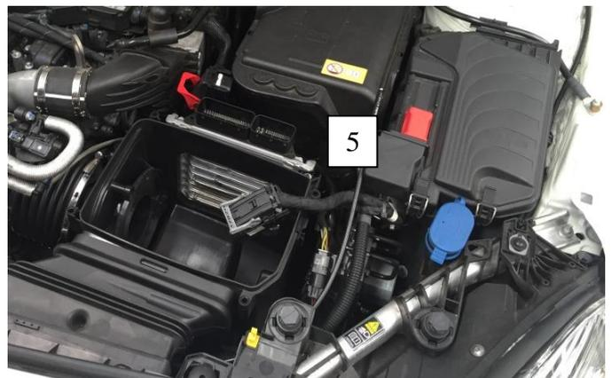
6. Unplug the pressure sensor on the left hand side of the air filter housing.
