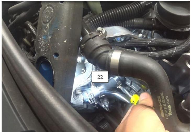
23. Install the supplied vacuum hose onto the fittings as required. Use the supplied spring clamps to secure the vacuum hose onto the fittings.
