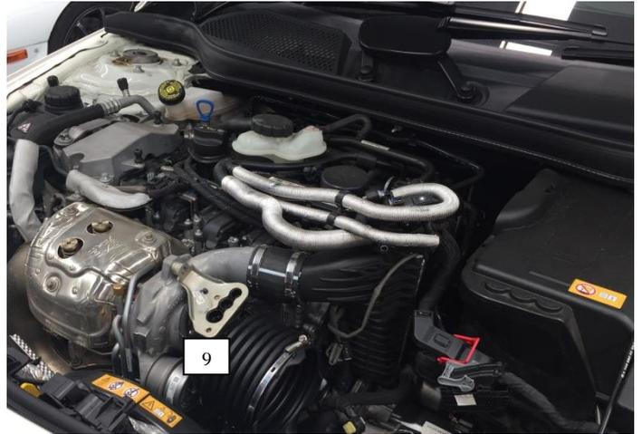
10. Undo screw/bolt attaching the turbocharger compressor cover to the ventilation hoses bracket.
