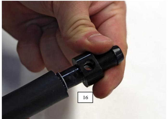
17. Install one of the supplied slotted hose clamps on the hose.
