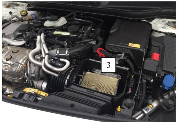
4. Detach the electrical connection from the air filter housing and place to one side.
