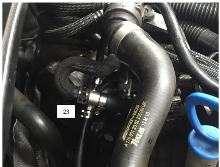
24. Route the vacuum hose towards the BOV location. Use the supplied cable ties to secure the vacuum hose in place. Ensure that the vacuum hose is not kinked or pinched.
