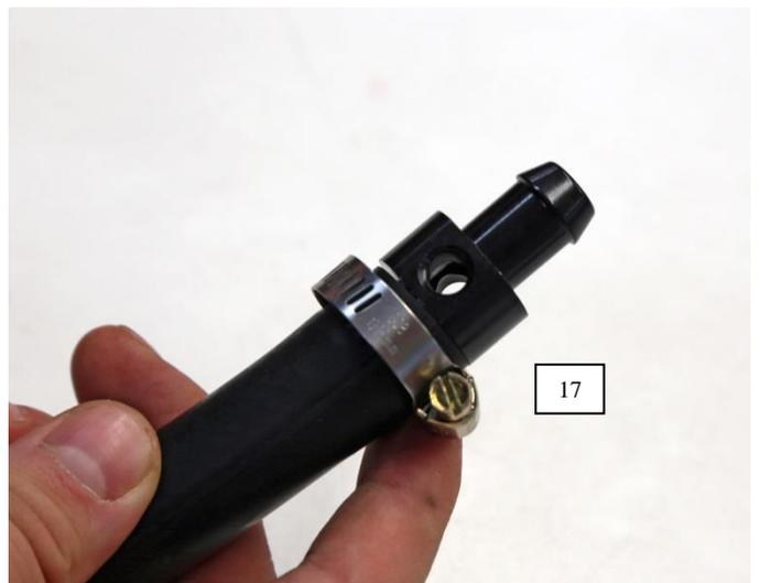
18. Install the supplied fittings as required. Use the larger nipple for the BOV. The smaller nipple is used for accessories such as boost gauges and boost controllers. Blank any unused ports with the provided blanking plug. Apply thread sealant as shown.
