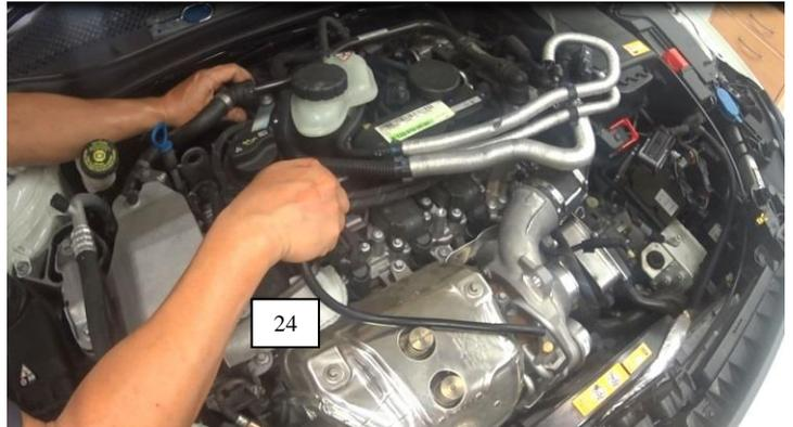
25. Install the other end of the vacuum hose on the BOV nipple. Use the supplied spring clamp to secure the vacuum hose on the nipple.
