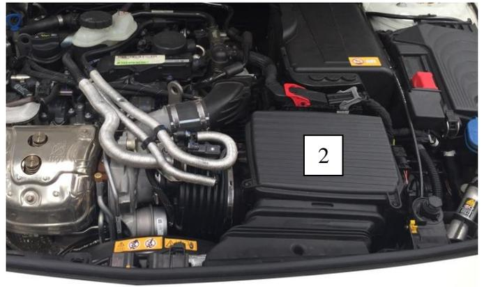
3. Remove the air filter by turning it towards the front of the vehicle (anticlockwise).
