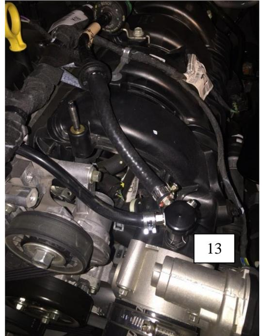
14. Locate the factory BOV and unplug the solenoid plug.
