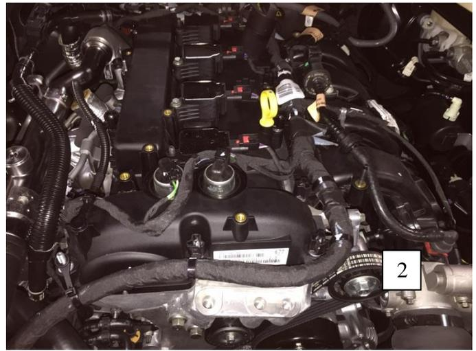
3. Install the included plug on the unused port of the boost reference adapter. **Apply thread sealant on threads.**
