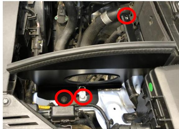
**Step 2:** Fit the airbox by inserting the inlet side into the hole in the mounting bracket then insert the filter neck into the existing intake hose, this can be secured by tightening the hose clamp. The Final bolt can then be tightened.
