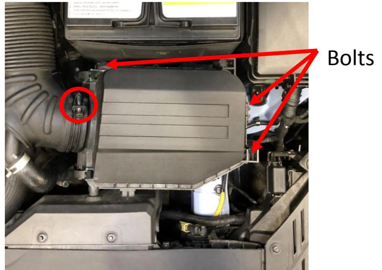
**Step 2:** Pull the hose off the left hand side of the airbox and remove airbox from the vehicle. The cold air feed at the base of the airbox will pop off when the airbox is lifted out.
