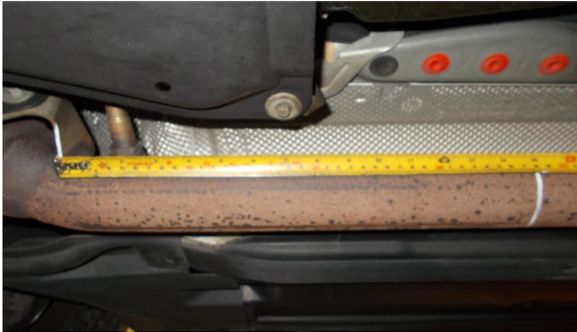
When fitting the Scorpion secondary de-cats the original system requires cutting in a specific place.
