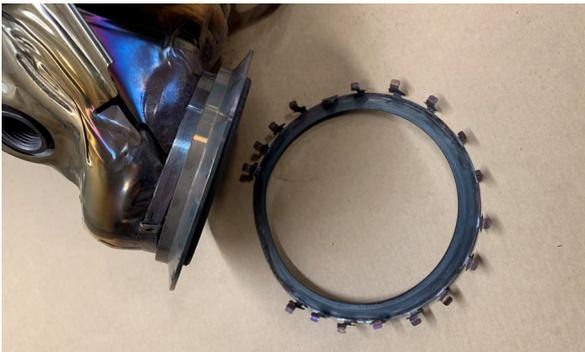
Remove the original gaskets from the original downpipe as they are required when fitting the Scorpion downpipe.
