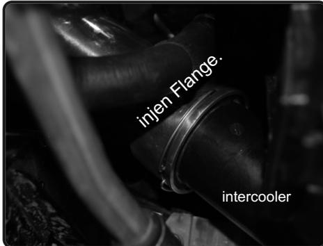
**25.** Slide the new charge pipe on the the intercooler. Locate the notch on the flange. Push until you hear a click. Once seated properly, pull back and tug on pipe to make sure the flange is secured and locked.
