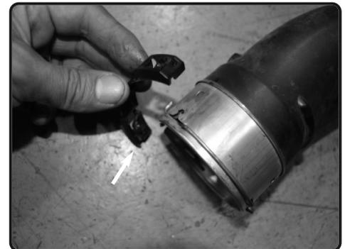
**16.** Pull of the plastic clip on the lower part of the plastic charge pipe.
