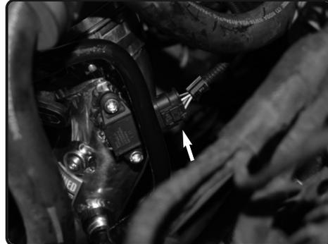
**30.** Re-connect the temperature sensor harness.
