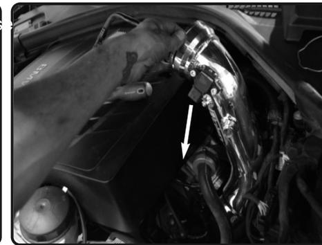
**27.** Install the upper charge pipe assembly into the vehicle and position to the lower part of the charge pipe.
