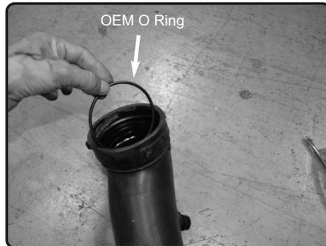
**14.** With a small flathead screwdriver, carefully remove the upper OEM O Ring out of the vehicle.
