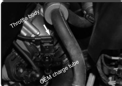
**9.** Pull back the charge pipe from the throttle body.
