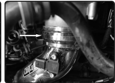
**28.** Install to the throttle body, push until you hear a click. Once seated properly, pull back and tug on pipe to make sure the flange is secured and locked.
