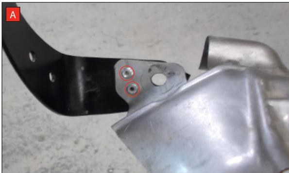
A) Prior to removing the original downpipe the heat shield needs to be removed. The black bracket on the heat shield is no longer required. Disconnect this by drilling out the two rivets circled in the picture.
