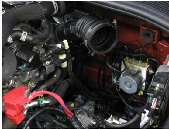
With the hose repositioned you can now drop the airbox in place, insert the filter outlet into the turbo hose, tighten up the hose clip and strap down the nose of the airbox.
