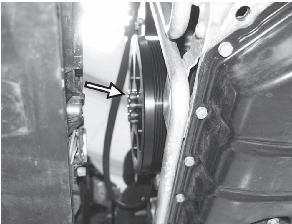
23) Place the APR pulley over the stock crankshaft pulley on the engine. Make sure that the offset hole in the APR pulley aligns with the offset hole in the stock pulley.
