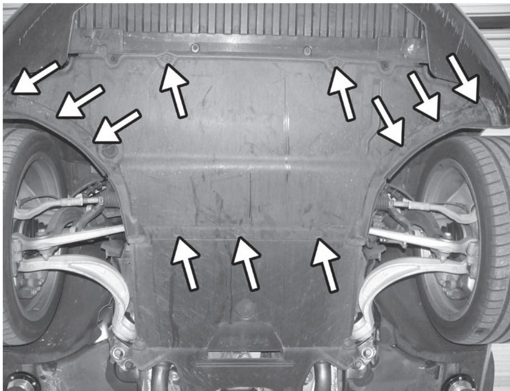
45) Install the 11x quarter turn fasteners onto the belly pan with a screwdriver.
