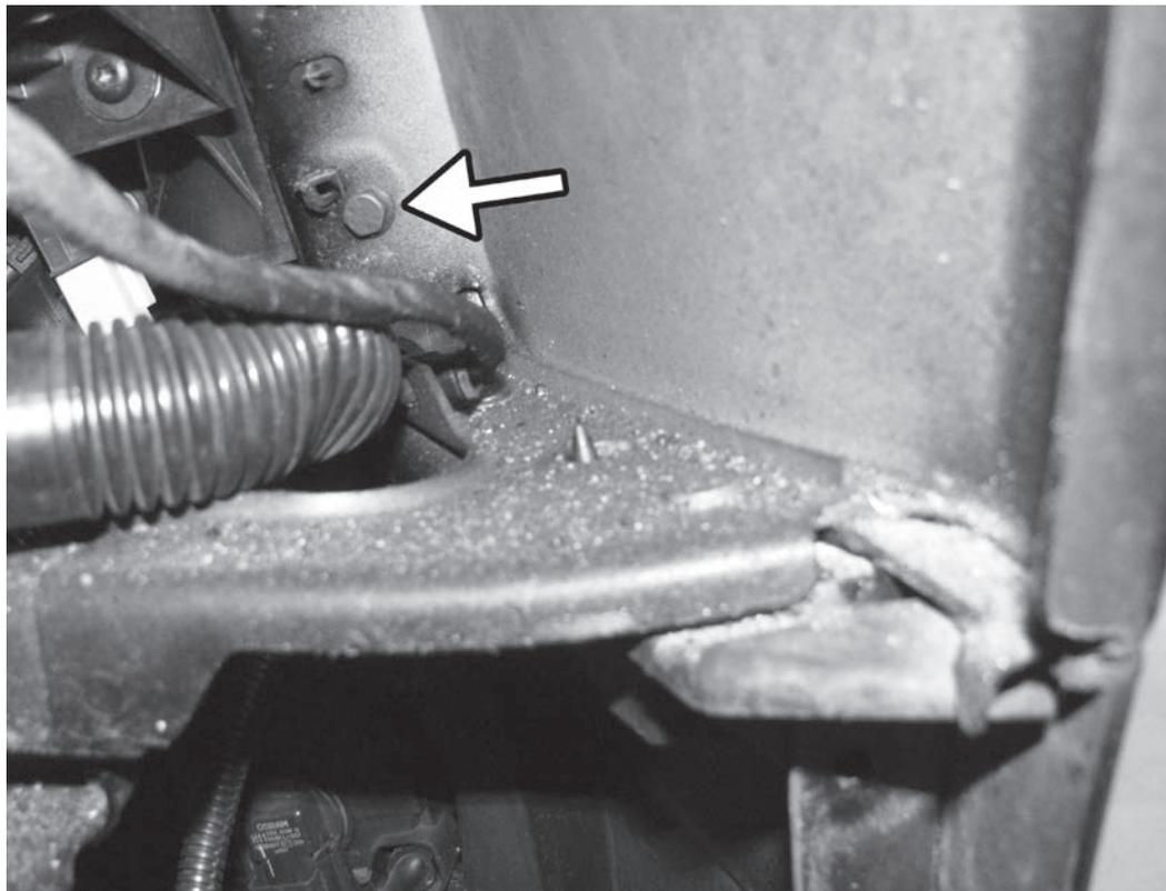
5) Pull back fender liner and remove the 10mm bolt from bumper cover. Repeat on both sides.
