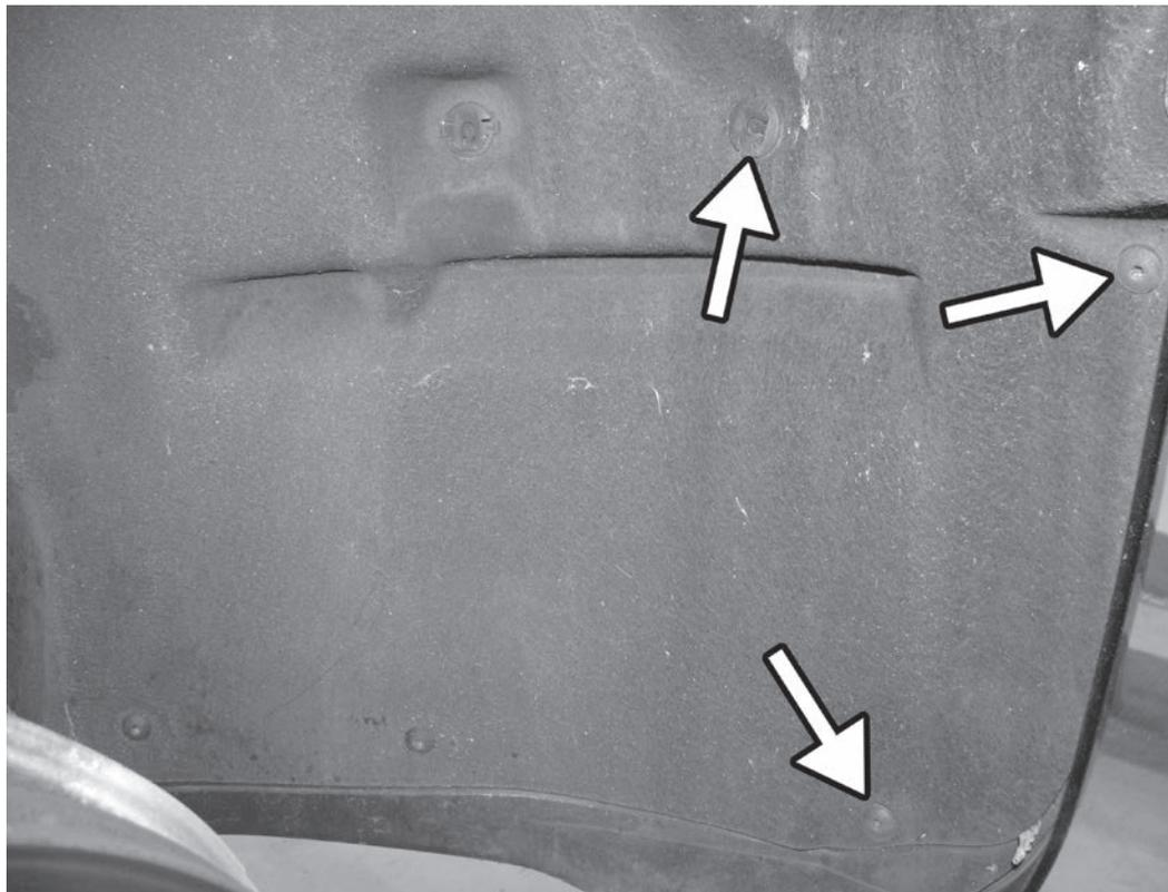
43) Reinstall the 2x outer T25 Torx screws from fender well liner and the outer plastic clip. Repeat on both sides.
