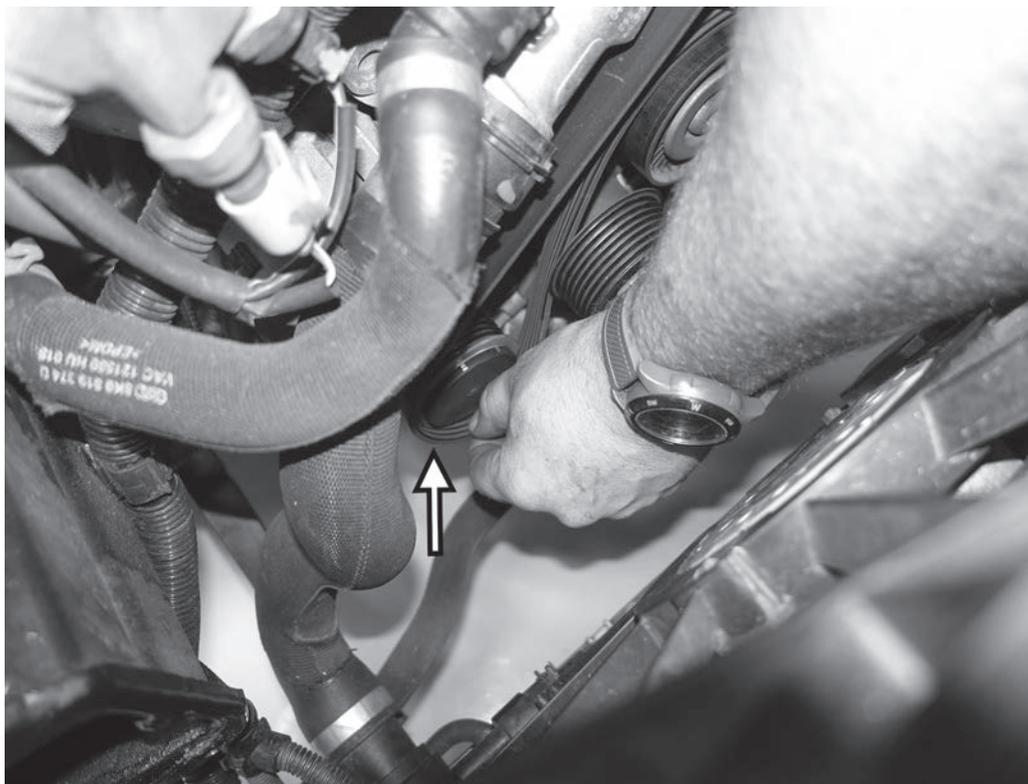
29) Reinstall the accessory belt by using a 17mm wrench to push down the accessory belt tensioner, and then slip the accessory belt over the alternator.
