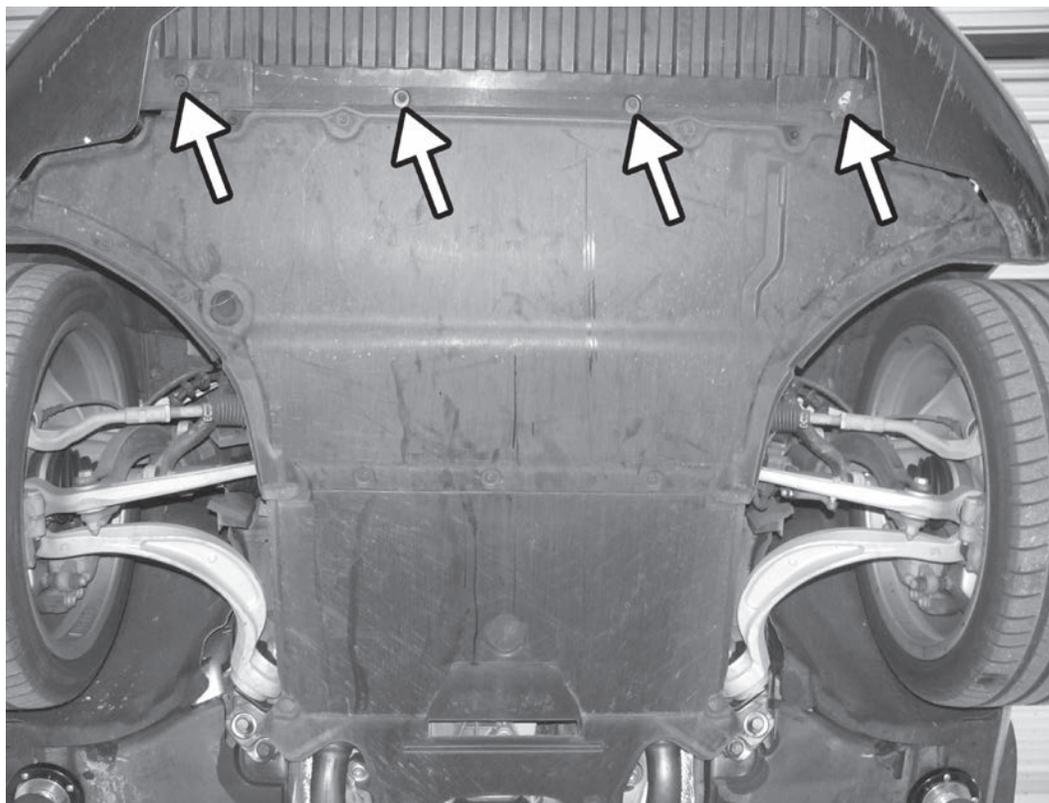
3) Remove the 4x T30 Torx screws from bottom of bumper cover.
