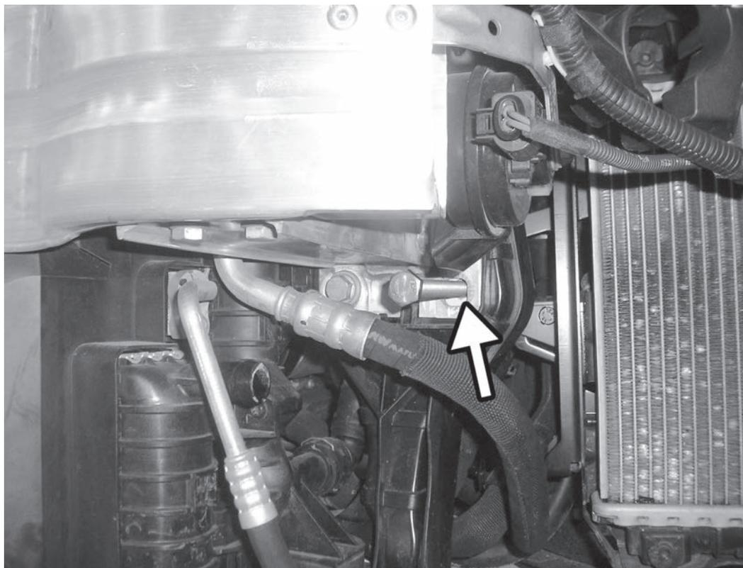
13) There are six 16mm bolts attaching the radiator core support to the front frame rails. ONLY remove the lower, outer bolts on both sides and replace these with the long bolts supplied with the APR Pulley kit. Only thread the bolts in to the same depth as the factory fastener.
