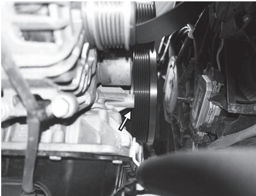
25) Observe how this post on the front of the engine block, just to the right of the crank pulley, is in the path of the supercharger belt by a few millimeters.
