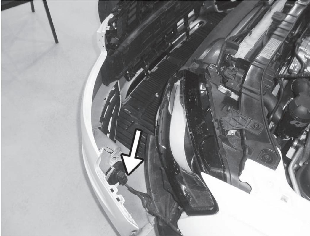
39) With an assistant, place the bumper cover back in front of the car. Reconnect the left and right fog light harness and bring the bumper back to its resting place on the core support.
