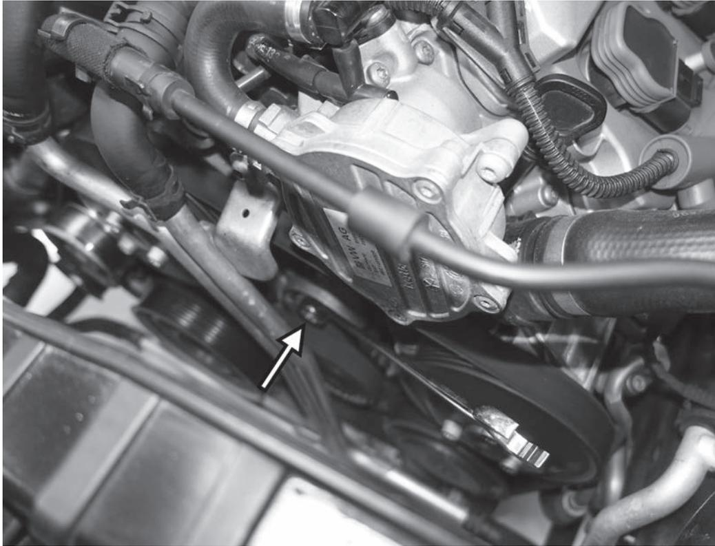
19) Using a 17mm wrench, loosen the tension on the accessories belt by pushing down on the wrench. With tension removed, slip the belt off the alternator pulley on the right side of the engine.
