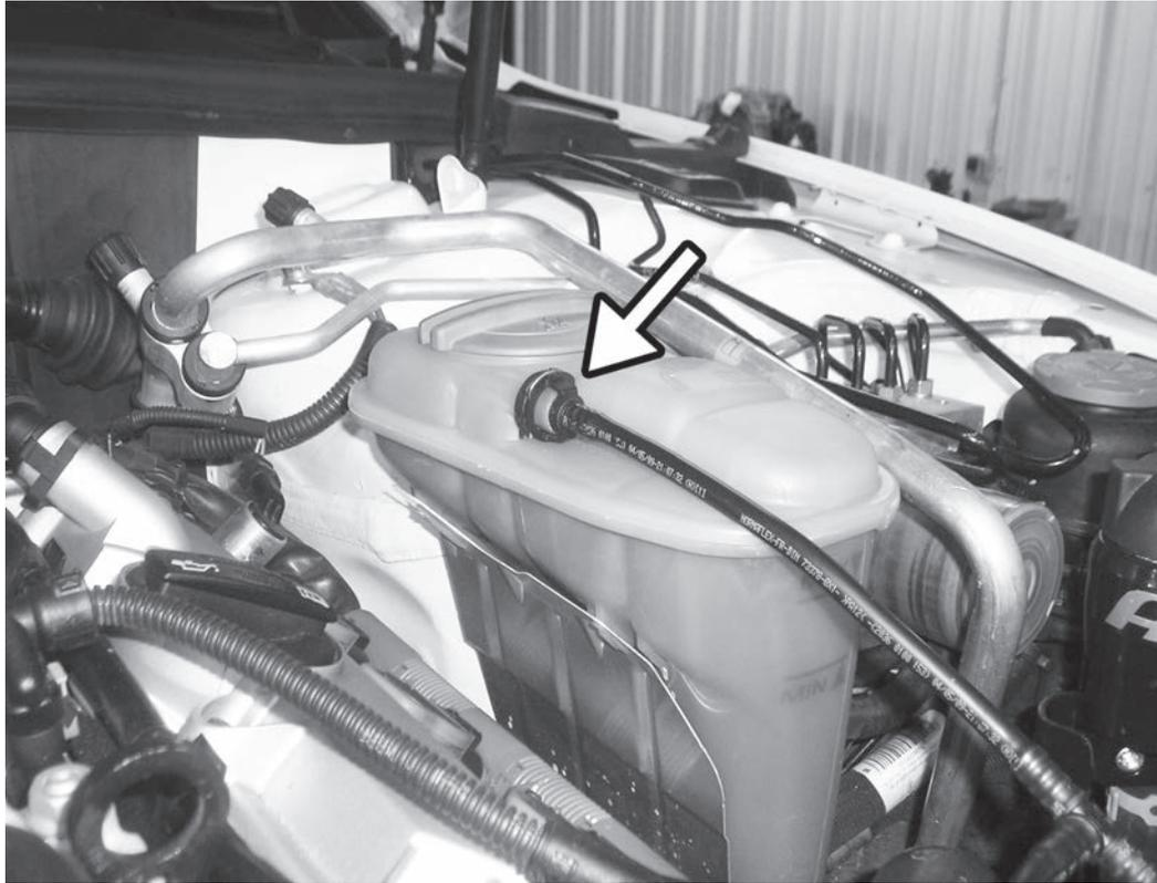
33) Reconnect the coolant hose to the front of the coolant reservoir.
