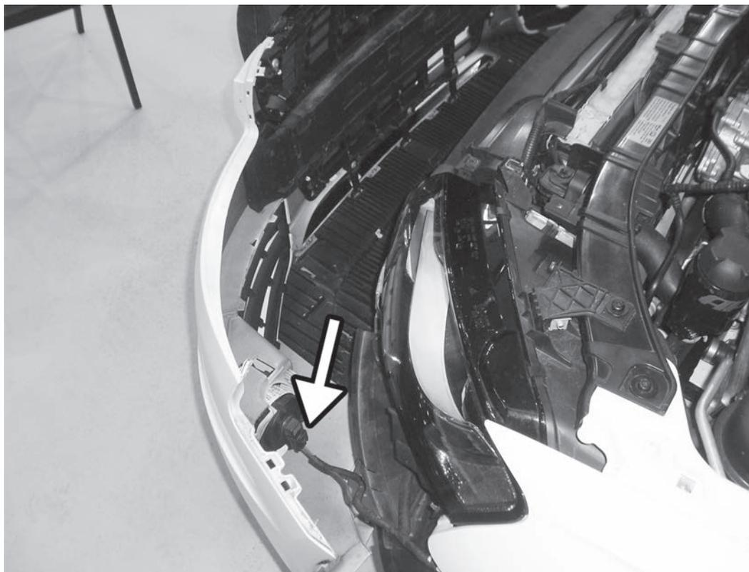
9) Carefully pull bumper cover forward and disconnect left and right fog light harness. Remove bumper cover.
