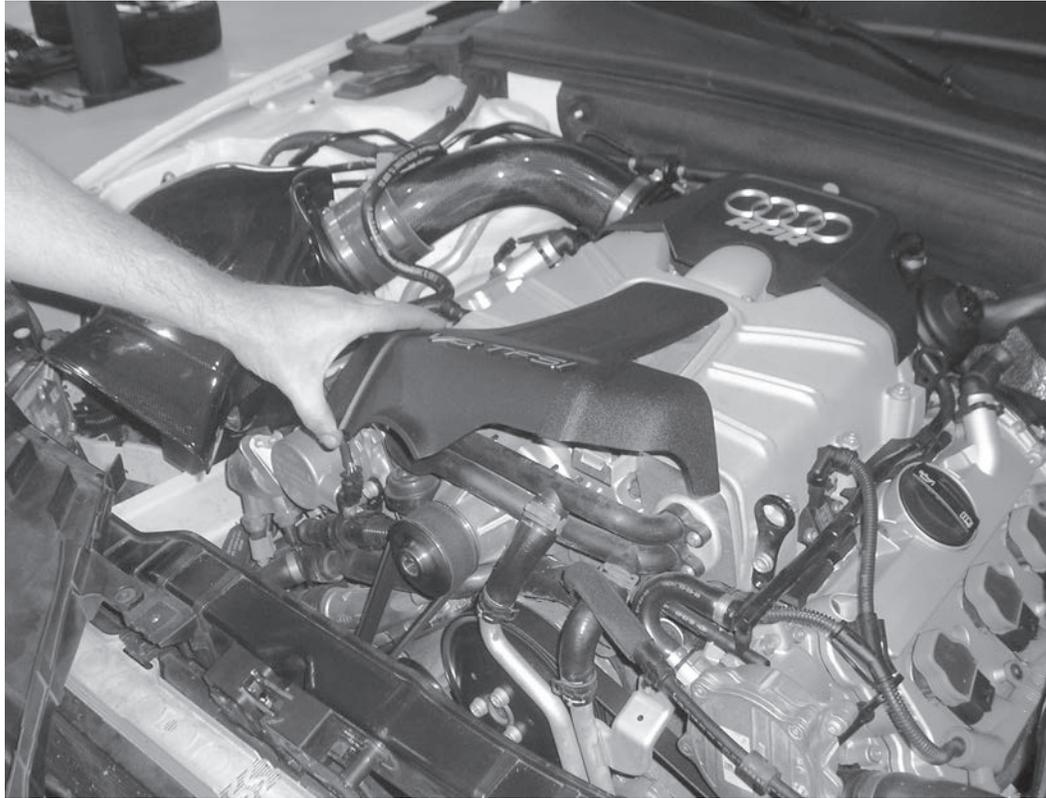
17) Remove front plastic cover from supercharger.
