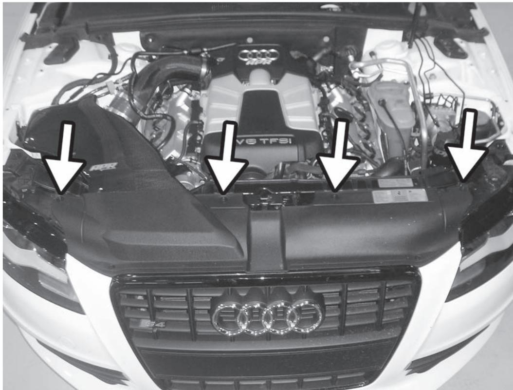
41) Reinstall the upper radiator trim cover with the 4x T30 Torx screws.
