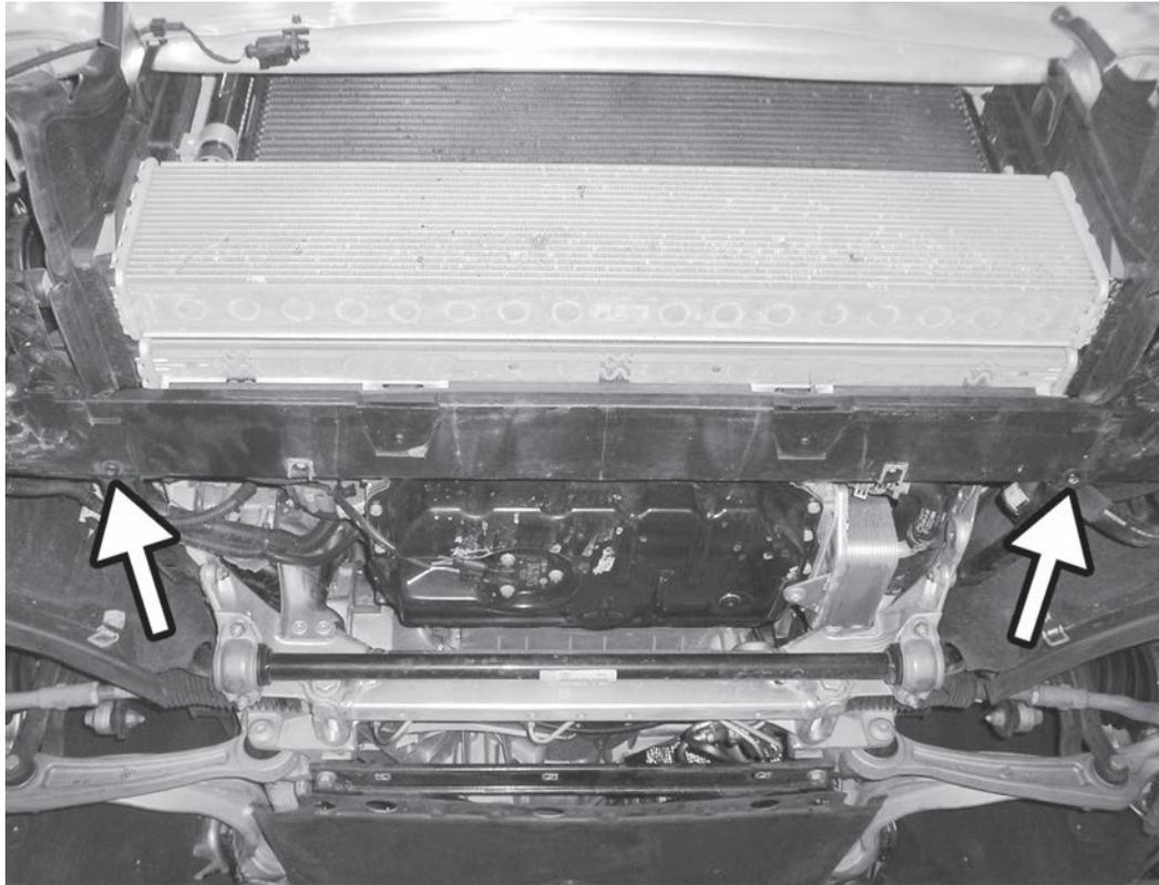
11) Remove 2x T30 Torx screws from bottom of radiator core support.
