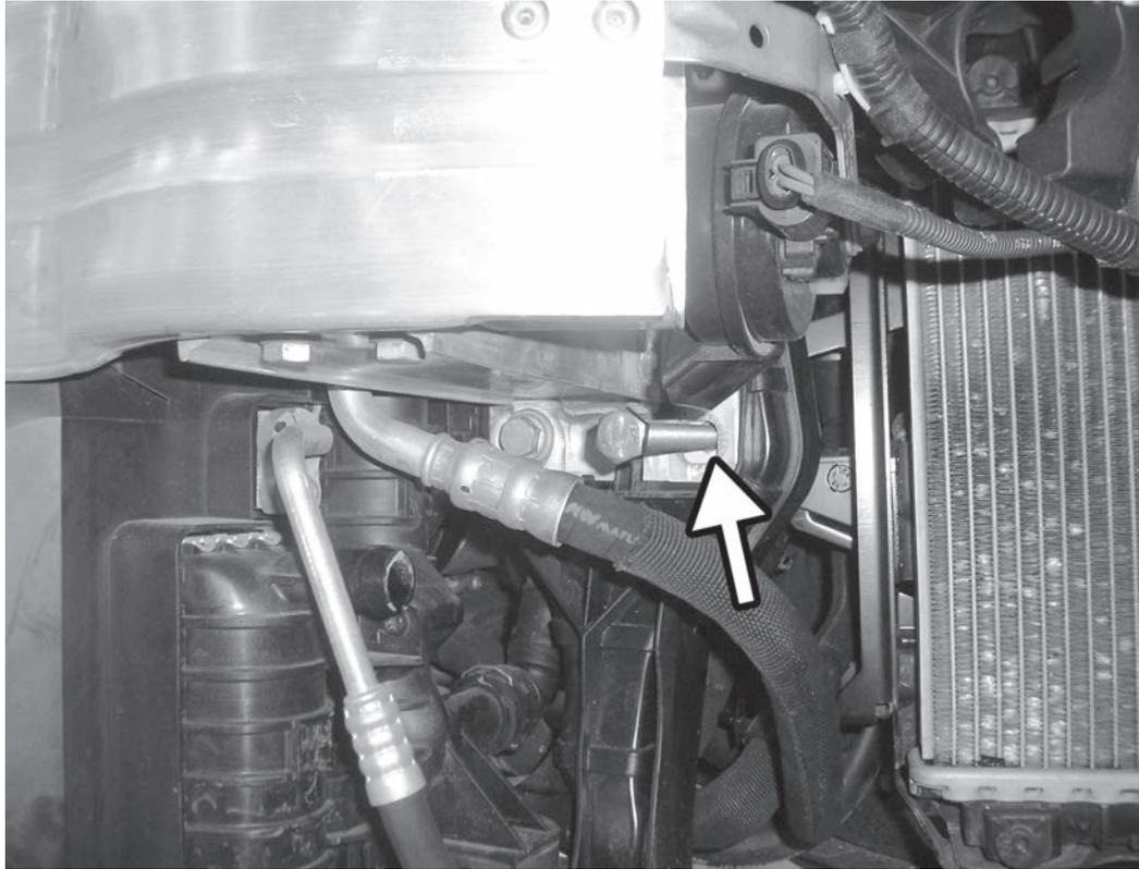
35) Remove the two long, supplied bolts and install the two remaining 16mm factory bolts in the frame rails. Tighten all six 16mm bolts holding the core support to the frame rails.
