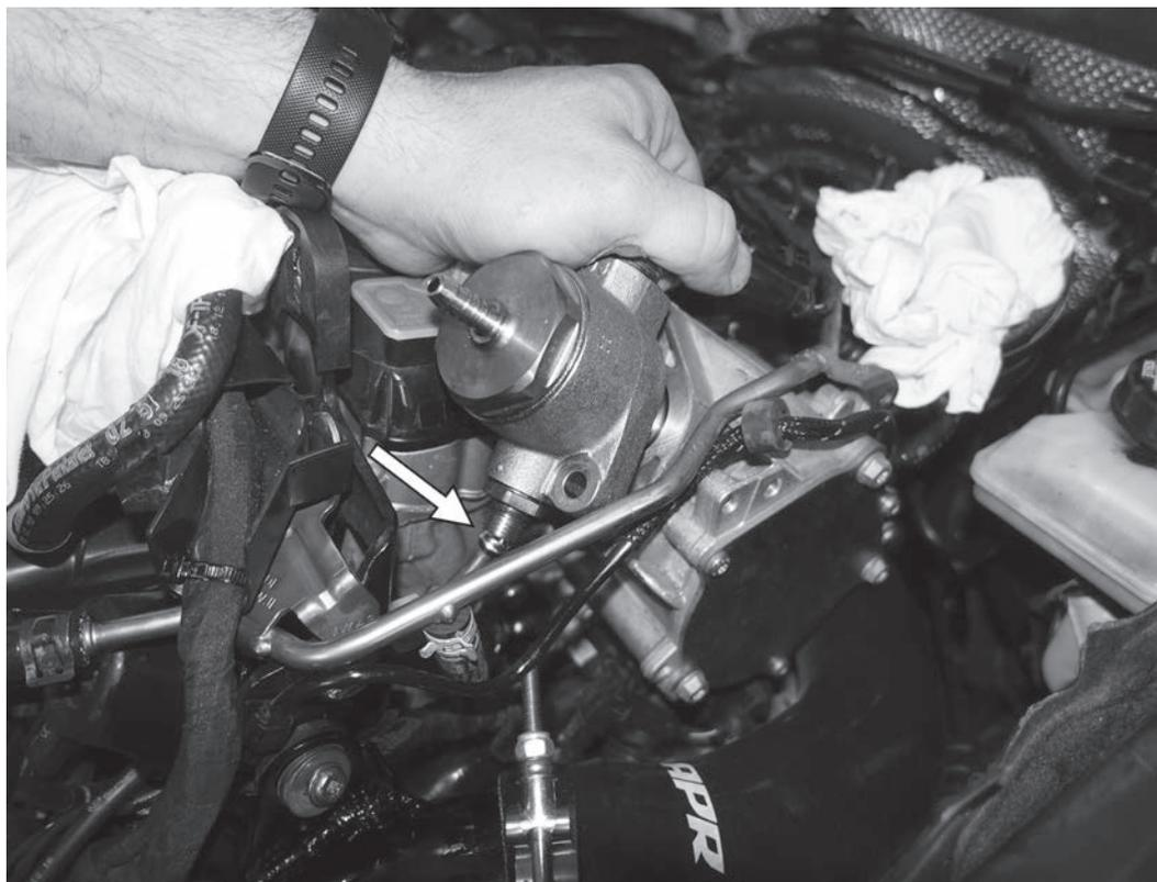
9) Pull the HPFP away from the engine just enough to pull the o-ring out of the housing in the cylinder head. Then, rotate the HPFP counter-clockwise to separate the pump from the outlet pipe. Remove the pump from the car. It is not necessary to remove the roller tappet from inside the cylinder head.
