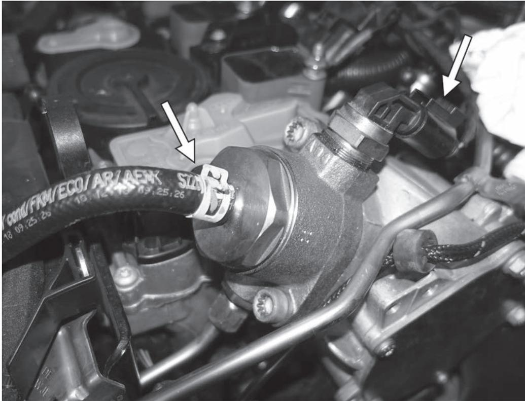
13) Reconnect the electrical connector to the solenoid on the top of the APR HPFP. Reinstall the fuel feed line to the front of the APR HPFP, and secure with the original spring clamp.
