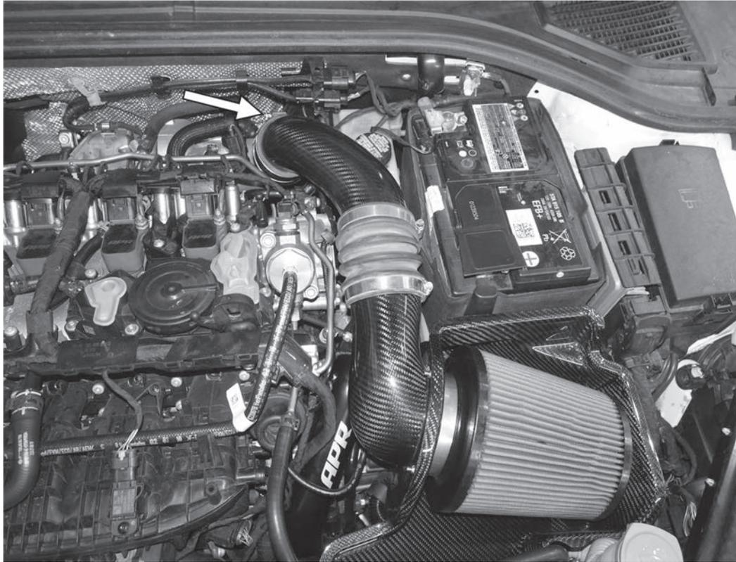
17) Place the intake back in the car, reconnecting the vacuum line to the bottom of it. Be sure all three mounting grommets are in place. Tighten the clamp holding the back of the intake to the turbocharger inlet. Finally, reinstall the engine cover.
