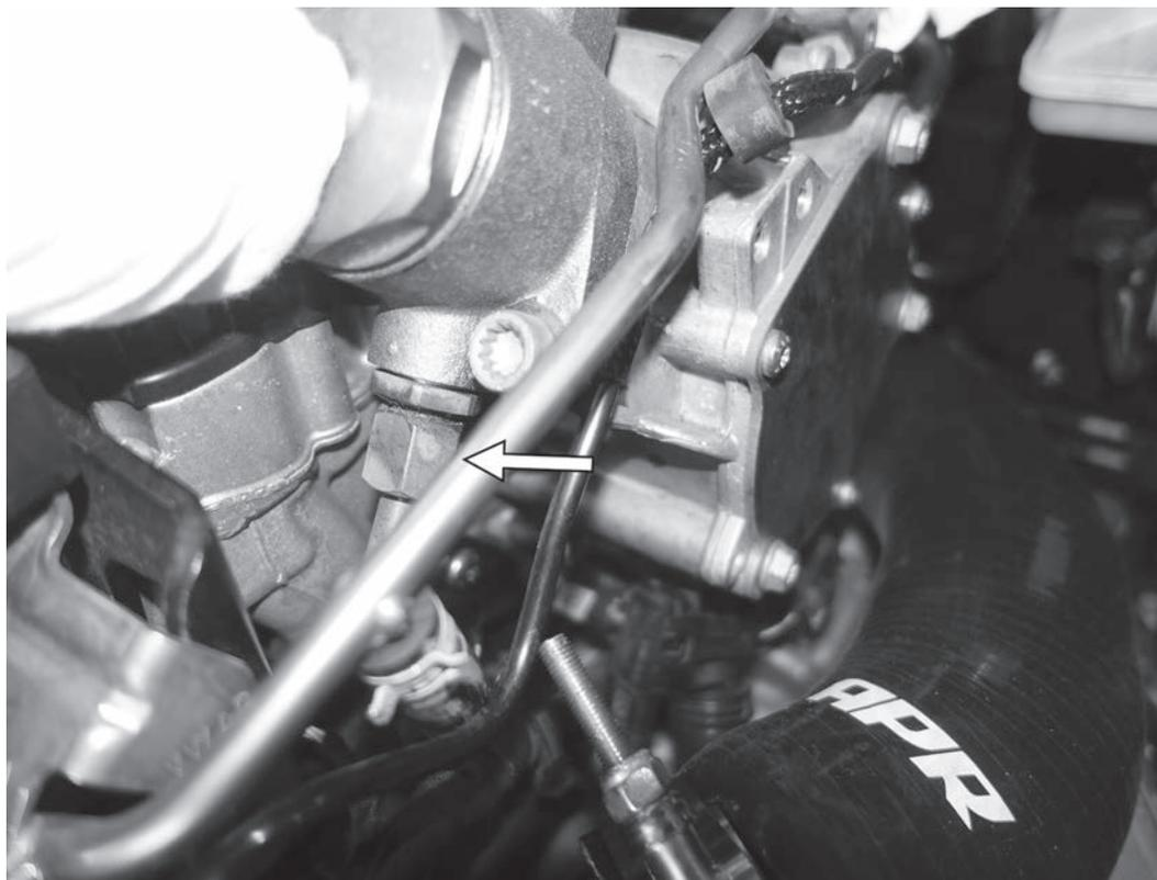
7) Loosen the 17mm nut from the HPFP outlet pipe. Some fuel will drain from here was well.
