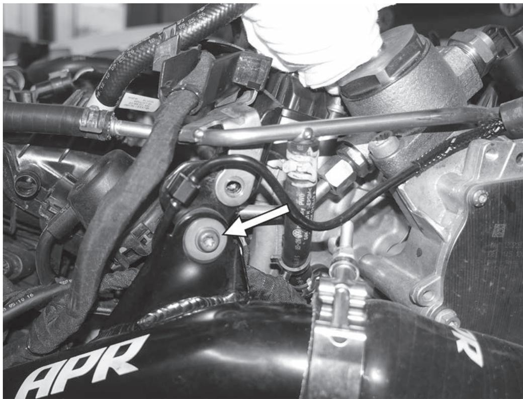
15) Reinstall the T30 screw holding the charge pipe to the intake manifold. Tighten this screw to 7Nm (62in-lbs).
