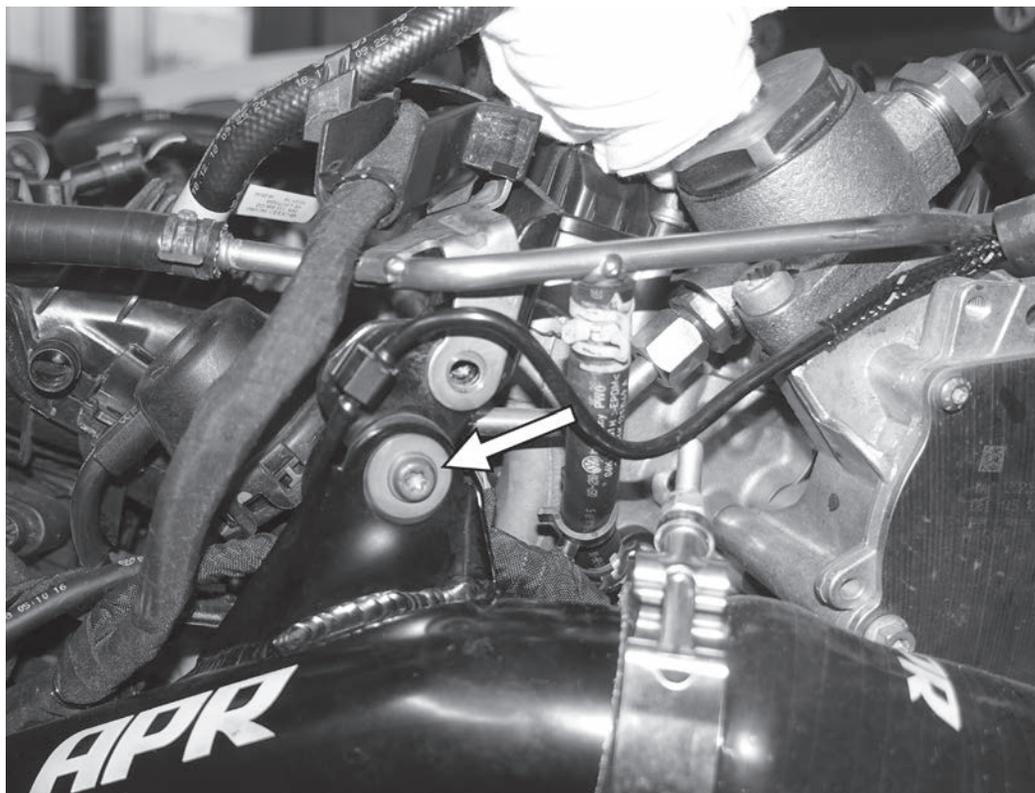
5) Remove the T30 screw from the side of the turbo outlet pipe.
