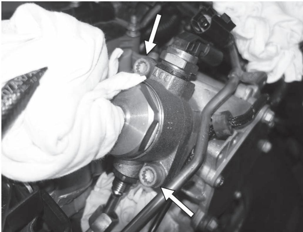
11) Ensure the outlet pipe sits correctly into the connection on the bottom of the APR HPFP. Install the two 10mm triple square screws and tighten to 20Nm (177in-lbs).
