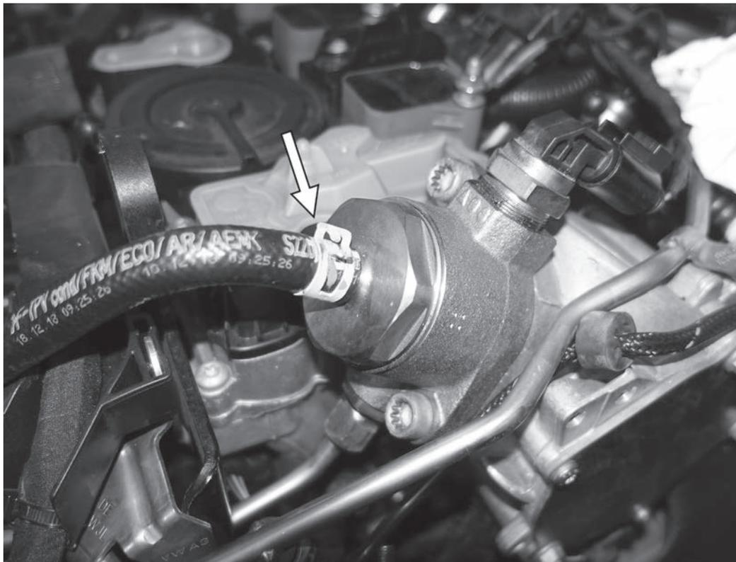
3) Remove the spring clamp from the end of the fuel feed line. Wrap the hose and connection with a rag before pulling the hose off of the pump, as gas will drain and can spray from the port in the HPFP.
