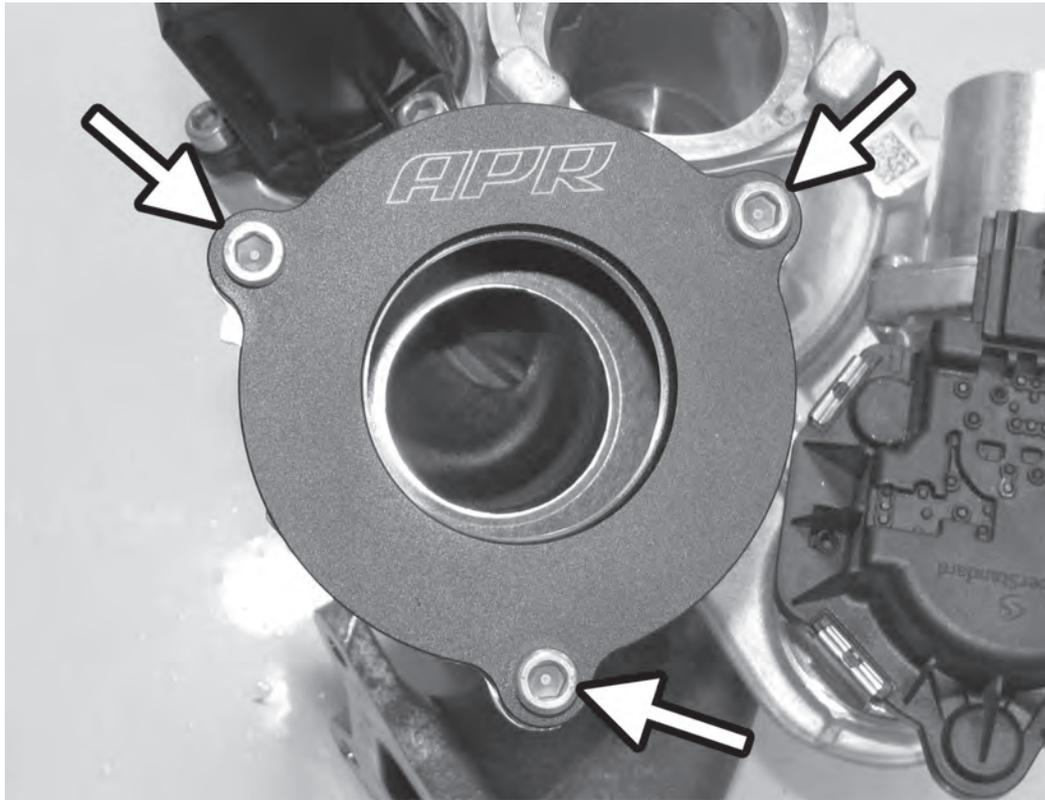
9) Reinstall the factory o-ring onto the turbocharger. It may be necessary to use some silicone o-ring grease to hold the o-ring in place. Install the outer ring of the APR muffler delete to the turbo with the three original 5mm allen screws. Make sure the o-ring is not pinched before fully tightening the three 5mm allen screws.
