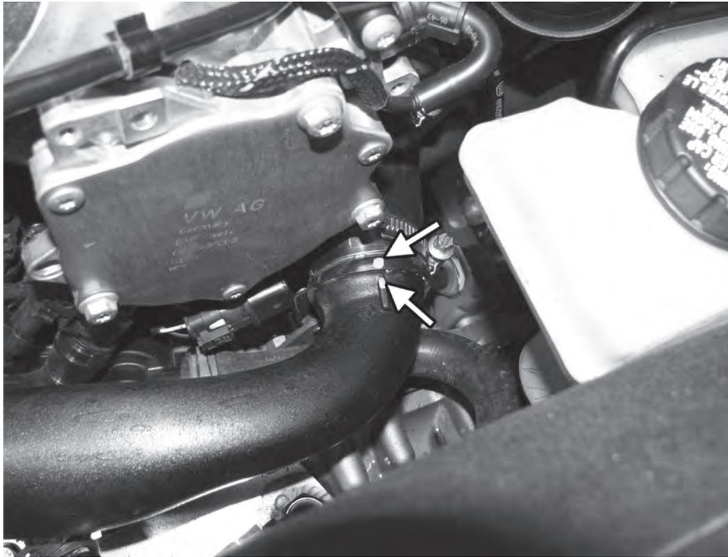
3) With a paint marker or grease pen, mark the orientation of the compressor outlet hose to the compressor outlet pipe on the side of the engine. Be sure to mark both sides.
