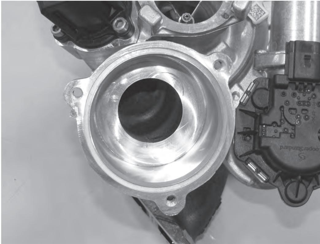
7) Remove the stock turbo muffler from the car. Be sure to remove the o-ring that seals the muffler to the turbo. Do not drop the o-ring in the turbocharger inlet.
