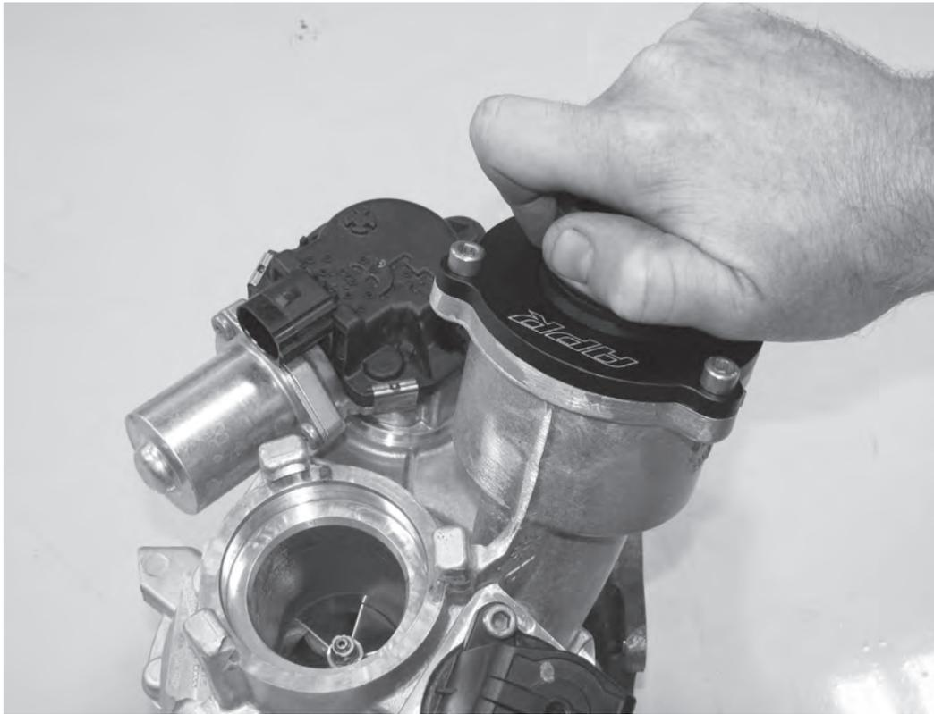
11) Firmly tighten the center section to the outer ring of the APR muffler delete by hand. The center section should compress the APR seal against the bottom of the stock muffler housing.
