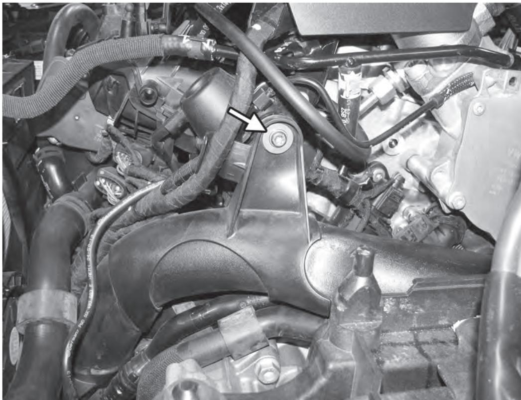
5) Remove the T30 screw from the side of the compressor outlet pipe. Maneuver the pipe slightly out of the way to remove the compressor outlet hose.
