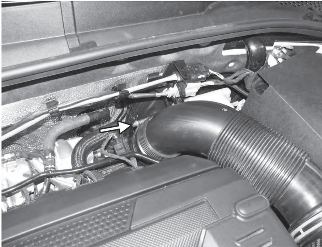
1) Loosen the hose clamp that connects the intake hose to the inlet of the turbocharger.
