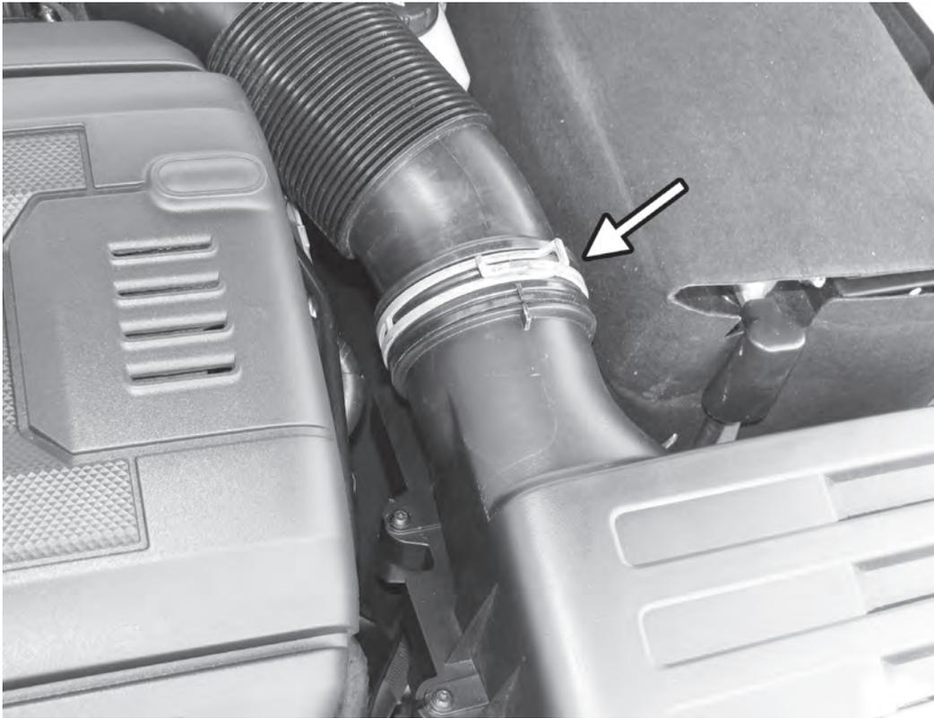
15) Reinstall the stock intake hose, connecting the spring clamp back to the airbox or intake on the car.
