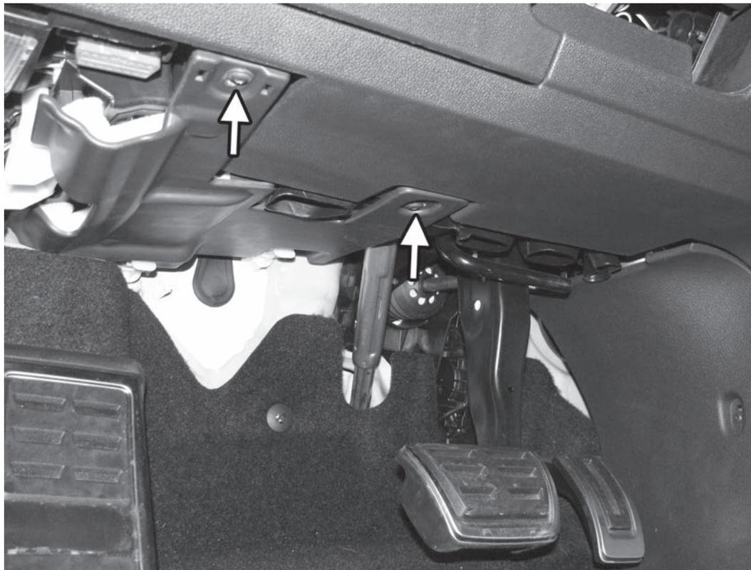
9) Remove the two T20 screws from the panel covering the bottom of the dash. Remove the panel by sliding it towards the back of the car.
