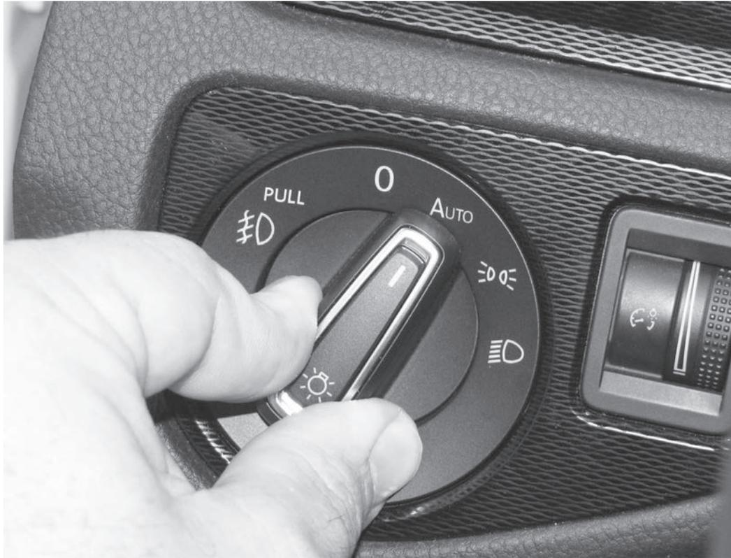
15) Remove the factory headlight switch. To do this, with the switch in the off position, simply push in on the switch, rotate the knob to the AUTO position. The switch can now be easily pulled away from the dash. Disconnect the red ten pin connector from the back of the switch. Do not turn on the ignition to the car with the switch disconnected.
