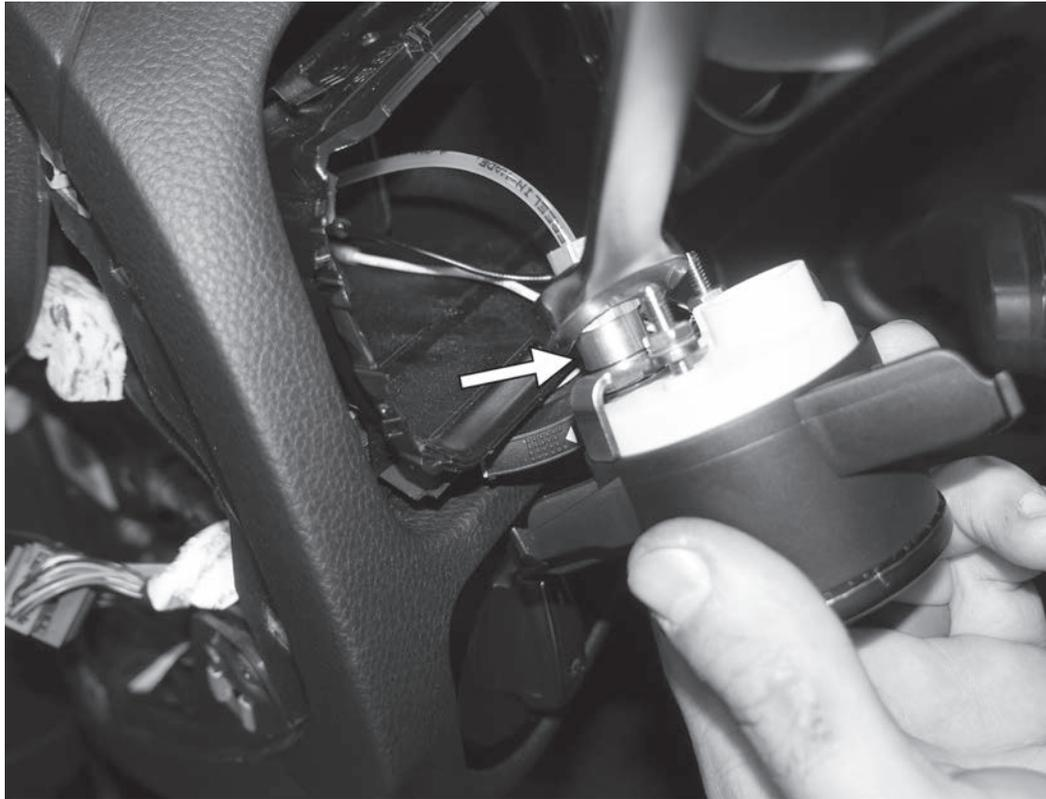
23) Connect the brass fitting from the nylon hose to the back of the preassembled boost gauge/pod, and tighten with a wrench.
