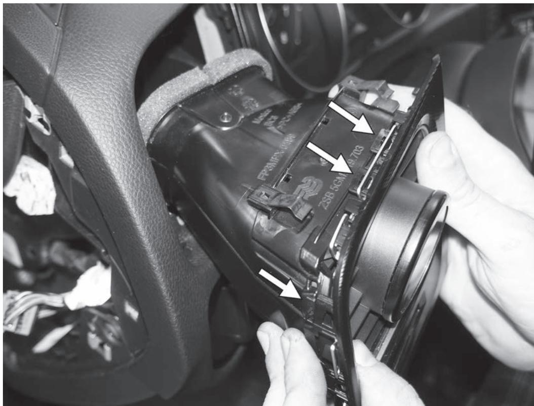
25) Slide the boost gauge with APR pod back into the back half of the factory air duct. Install the front face of the factory air duct, reclipping all eight of the factory clips in place.
