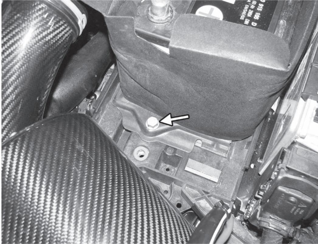
33) Slide the battery back on the battery tray. Slide the battery bracket back onto the battery, and reinstall the 13mm bolt to the battery hold down bracket.
