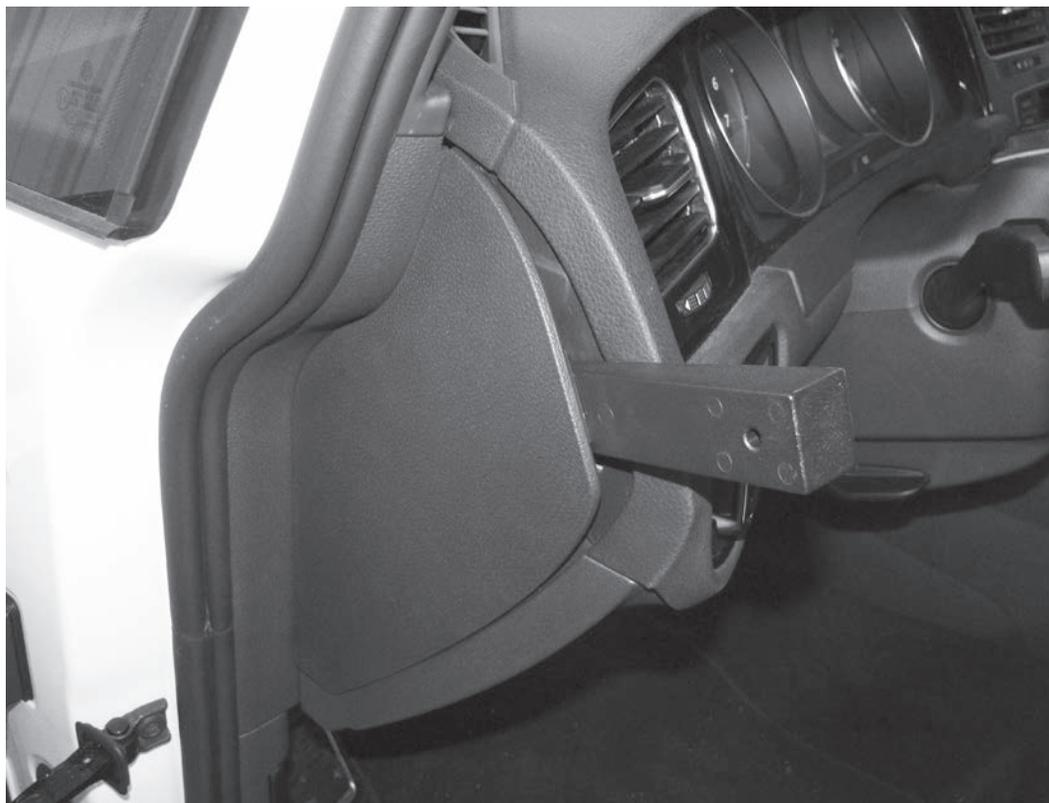
1) Using a plastic wedge or interior trim tool, remove the access panel inside the driver's door jam.
