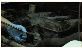
7. You will now be able to remove the stock thermostat. Once the thermostat is removed, use a scraper to remove any old, left over gasket on the thermostat housing.
