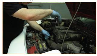
4. Reinstall the upper radiator hose, securing it with both hose clamps.
