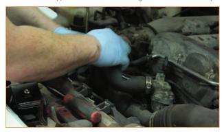
**5.** It is now time to refill the vehicle with coolant. Screw your coolant drain plug back in if you haven't done so already. Insert the funnel into the filler neck of the radiator and begin to pour in a 50/50 mix of coolant and distilled water. While filling, it is a good idea to pump the upper radiator hose to remove any last bit of air in the system.
