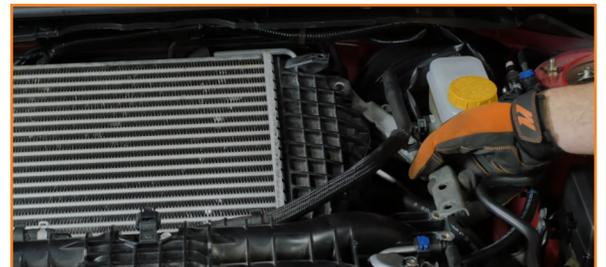
5. Lift the intercooler out of the engine bay.
