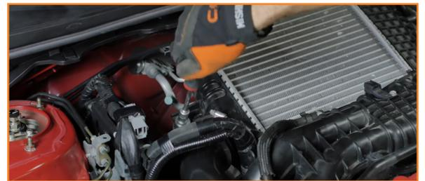
4. Remove the bolts on the intercooler bracket, located on the driver side. (2x 12mm bolts)
