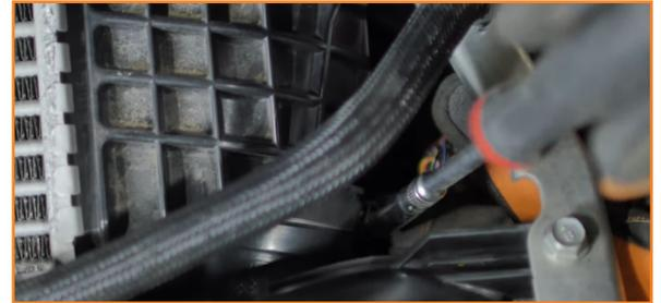
3. Remove the bolts that secure each side of the intercooler. (2x 12mm bolts)
