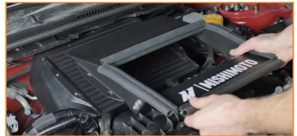
18. Install the shrouding to the face of the intercooler. Align the holes on the bracket with those on the intercooler. (4x 4mm Allen bolts)
