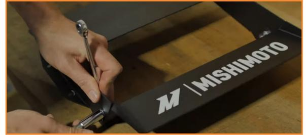
17. Attach the rubber pieces to the shrouding. The shorter pieces go on the sides and face outward.
