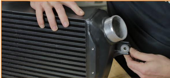
9. Install the Mishimoto intercooler. Angle the top of the intercooler in first.
