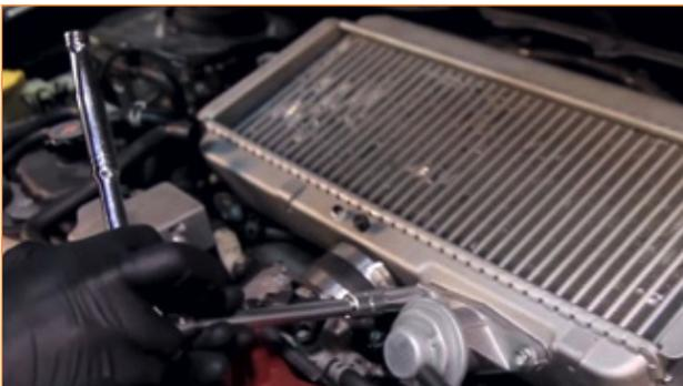
4. Remove the two driver-side bracket bolts on the intake manifold.
