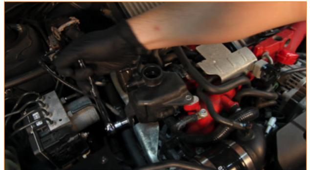
5. Remove the clamp hose from the bottom of the expansion tank. (1x clamp)
