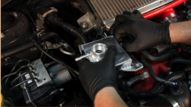
2. Reinstall the bolts on the expansion tank. (2x 12mm bolts)
