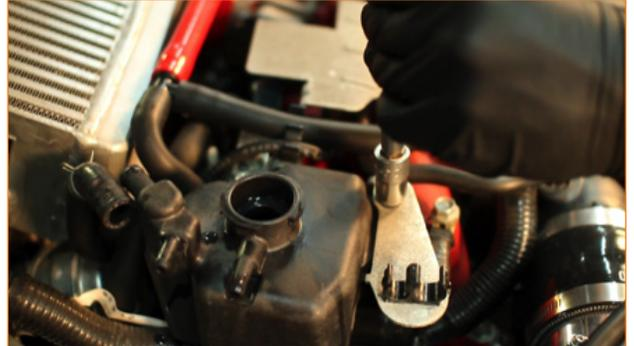
4. Remove the final nut holding the expansion tank in place. (1x 12mm nut)
