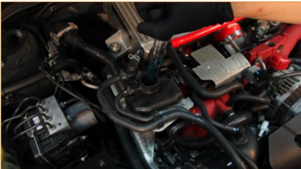
2. Remove the three ancillary clamps and hoses on top of the expansion tank. (3x clamps)
