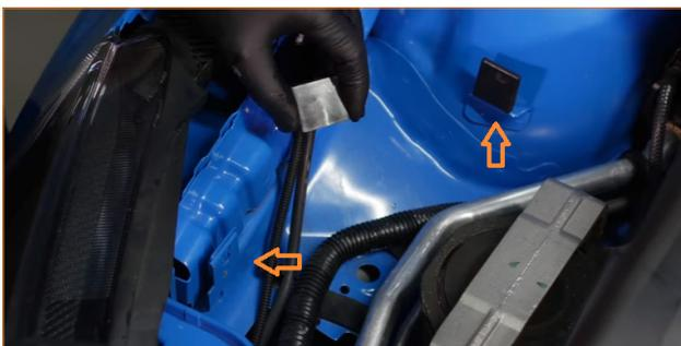
07. Remove the isolator from the bottom of the stock expansion tank, and transfer it to the Mishimoto expansion tank.
