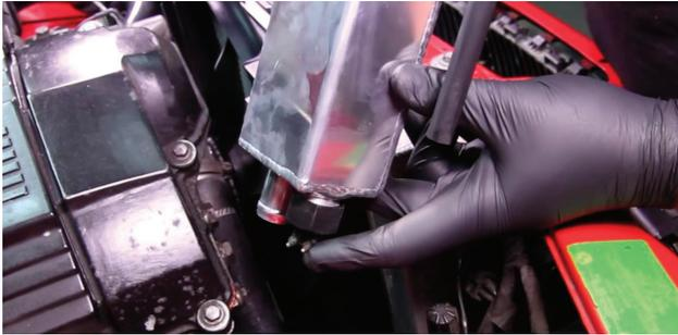
10. Install a worm-gear clamp over the lower coolant hose, and then slip the lower port on the Mishimoto expansion tank into the lower coolant hose. Tighten the worm-gear clamp to secure the hose. (1x worm-gear clamp)
