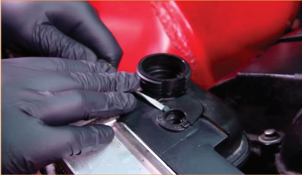
04. Loosen the worm-gear clamp connecting the expansion tank and the overflow hose. To locate the clamp, tilt the expansion tank toward the motor, and look through the hole from which the bleeder screw seal was removed. Pull the overflow hose off the expansion tank. (1x worm-gear clamp)
