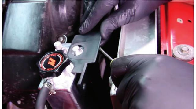
14. Reinstall the pop-clip that secures the top of the fan shroud. (1x pop-clip)
