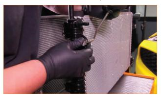
**22.** Transfer the final clip-nut from the mounting post on the stock radiator to the Mishimoto mounting post.
