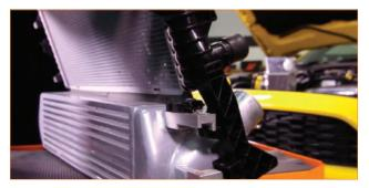
21. Remove four clip-nuts from the stock radiator and transfer them to the Mishimoto radiator. (4x clip-nuts)
