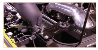
15. Loosen the clamps that secure the intercooler couplers to the intercooler. Then separate the intercooler couplers from the intercooler.
