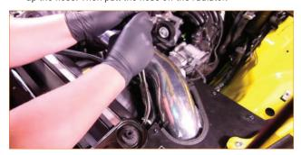
**06.** Compress the spring clamp that secures the rear coolant hose on the expansion tank and slide it down the hose. Then remove the hose from the expansion tank.
