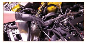
**07.** Remove the two 10mm bolts that secure the expansion tank to the fan shroud. (2x 10mm bolts)
