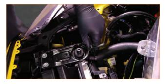
Disconnect the electrical harness for the cooling fan.
