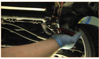
**5.** Using your ratchet, remove the two 10mm bolts securing the air conditioning line to the vehicle.
