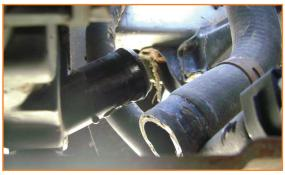
**Please Note** - If you have an automatic transmission, you will need to remove the transmission oil cooler lines. Keep in mind that late model Fords tend to use quick connect transmission oil cooler fittings and these require special removal. Research your engine to find out the proper method of removal of the transmission oil cooler lines.
