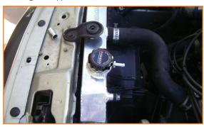
**4.** Fill radiator with coolant. Consult owner's manual for the proper mixture of antifreeze and water.
