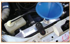
5. While the radiator cap is still off, bleed air in system by starting your car's engine and turn on the heat, continually topping off the radiator as bubbles work their way out. Be sure to squeeze the radiator hoses to help air exit the system. Use caution as you squeeze the hoses, as they will have become hot. Once you are satisfied that you have bled your system of air, replace the radiator cap.
