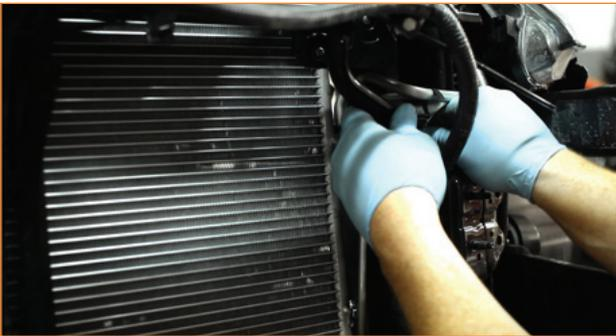
8. Now the upper radiator hose will need to be reinstalled. The original radiator used a plastic clip-in connector. The Mishimoto radiator eliminates this plastic connector with the use of a different hose outlet. To install the hose, separate the plastic connector from the rubber hose and place this directly on the Mishimoto hose outlet. Secure this hose with a clamp.
