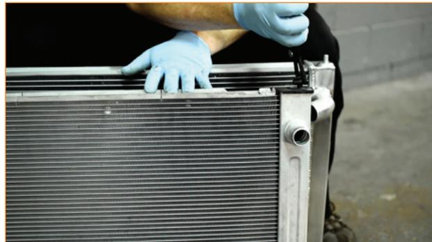
2. Remove the AC receiver drier from the OEM condenser, and install the drier on the Mishimoto condenser.
