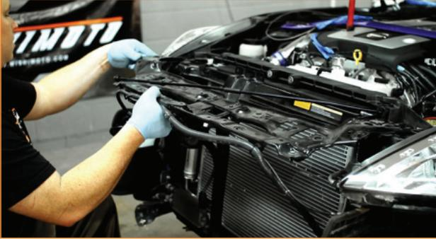
7. Reattach the hood latch and its bracket.
