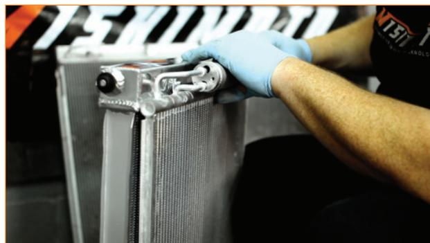
3. Place the assembled Mishimoto radiator into the vehicle. Be sure that the lower mounts fit into the proper position.
