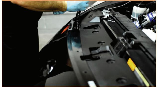
6. Remove the 10mm bolt located in each front fender well. These bolts secure the front bumper to the splash guard.
