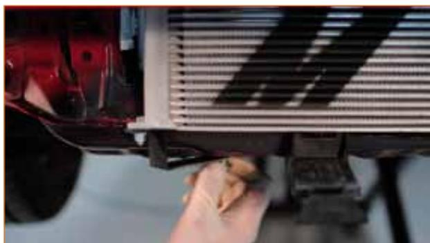
8. Install the shorter oil line to the left side of the cooler using the 150° fitting.
