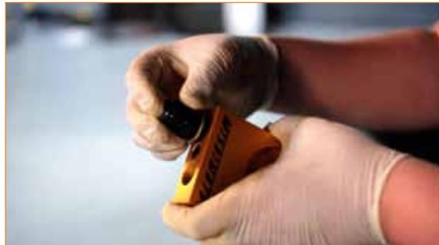
14. Lubricate the O-rings on the sandwich plate to ensure a proper seal.
