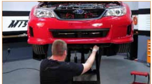
9. Remove the bumper. Pull out on the sides of the bumper to disconnect it from the clips.
