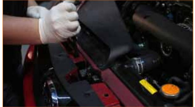
3. Remove the eight pop clips from the inside of the fender wells. There are four on each side.
