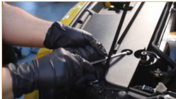
4. Remove the bumper hardware, but do not fully remove the front bumper yet. (4x pop clips – 2 located on each side, 6x 8mm screws)
