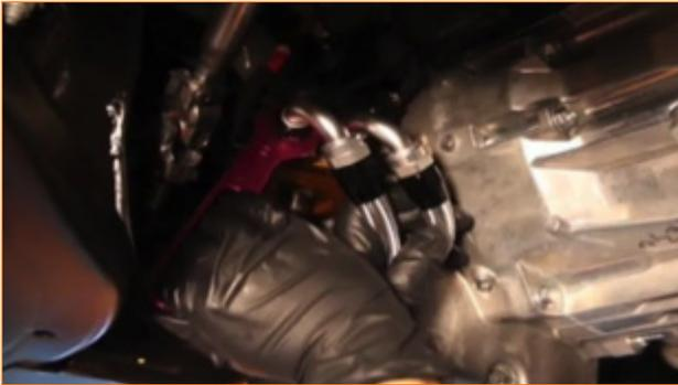
8. Lubricate the O-ring and, reinstall the oil filter.
