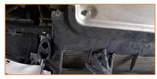
Loosen the bolts that secure the oil cooler brackets. (3x 13mm bolts)
