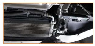
4. Remove the nuts that secure the lines to the oil cooler. (2x 10mm nuts)
