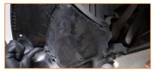
2. Remove the bolts on the center splash shield. (7x 8mm bolts, 2x 13mm bolts)
