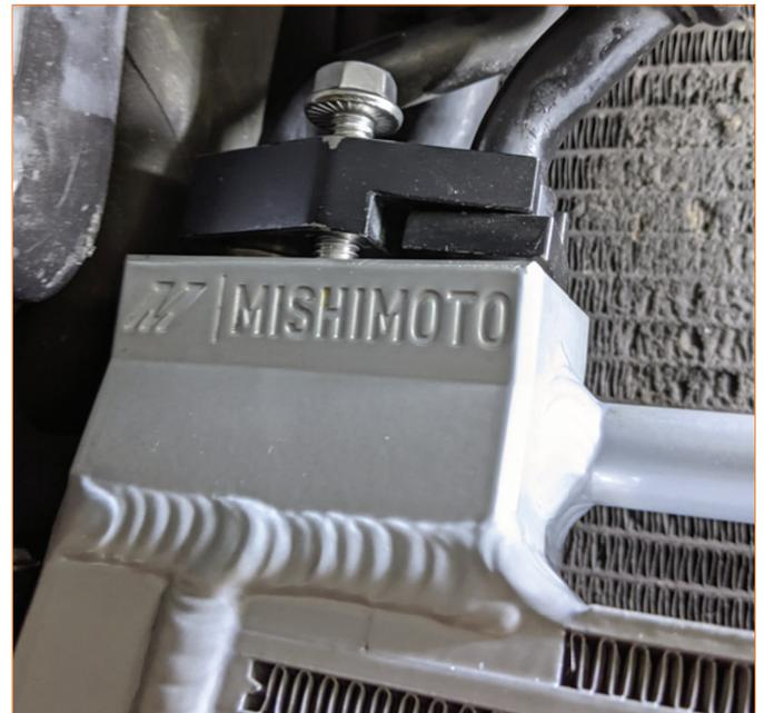
**Note: Be sure the oil cooler lines and O-rings are seated correctly**
