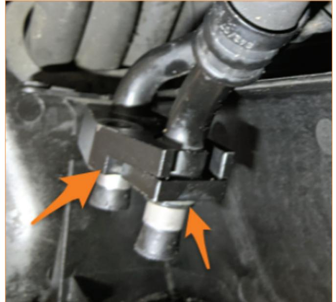
08. Install the oil lines onto the Mishimoto oil cooler with supplied bolt.
