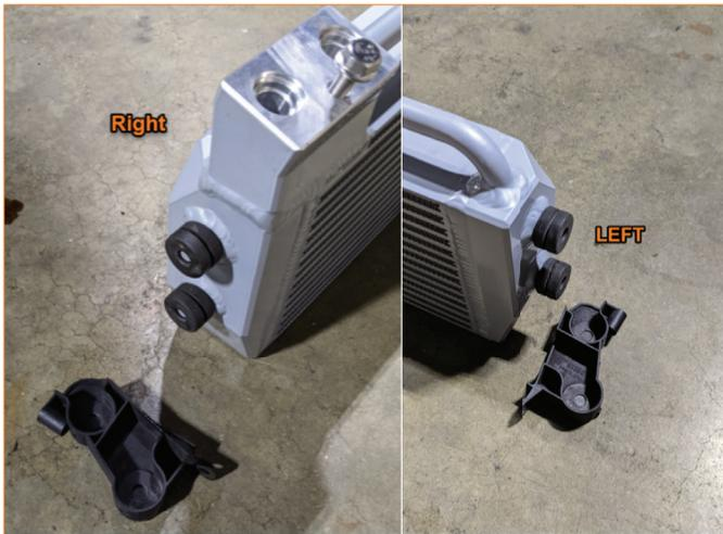
06. Install the Mishimoto oil cooler in the stock location, using stock hardware.
