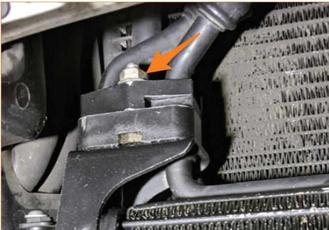
03. Remove the 4x torx bolts from the oil cooler hold down bracket. Be sure to take note which side each bracket is on and put aside. The stock plastic brackets will be used to reinstall the Mishimoto oil cooler.
