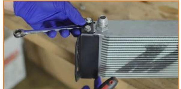
21. Install the oil cooler where the brake duct used to be. Use the longer bolts for this step. (2x 10mm bolts)
