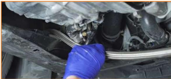
17. Install the 90° end on the shorter cooler line to the right-side port.
