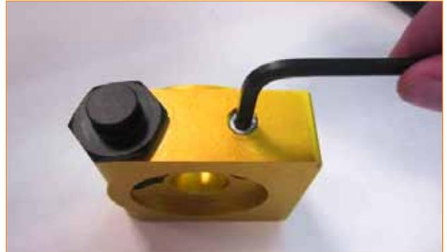
5. Remove any excess Teflon® after tightening.
