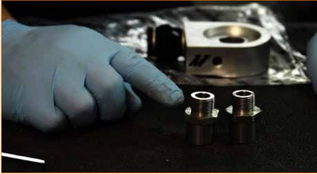
5. Remove oil filter and install sandwich plate to oil filter housing. Next, install appropriate adaptor in center of the sandwich plate. Tighten the adaptor in hold sandwich plate in place (27mm socket). Lastly, tighten the banjo fittings using the same 27mm socket.
