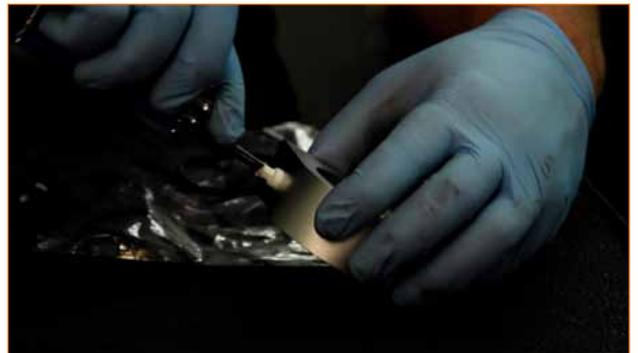
2. Install O-ring seal on sandwich plate.
