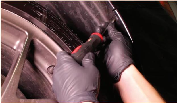
06. Release the bumper cover from its retaining clips by pulling it out from the corner. Do this on both sides.
