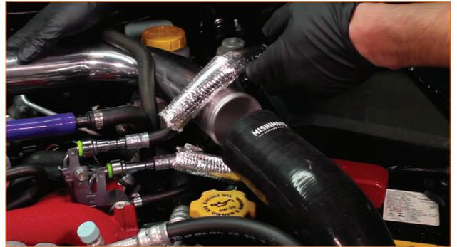
46. Locate the turbocharger outlet coupler. This coupler has an indentation. Slip a T-bolt clamp on each end, and install the narrow end onto the turbocharger. Insert the free end of the 90° pipe into the other side. (2x T-bolt clamps)
