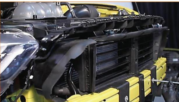
**36.** Reattach the ambient temperature sensor.
