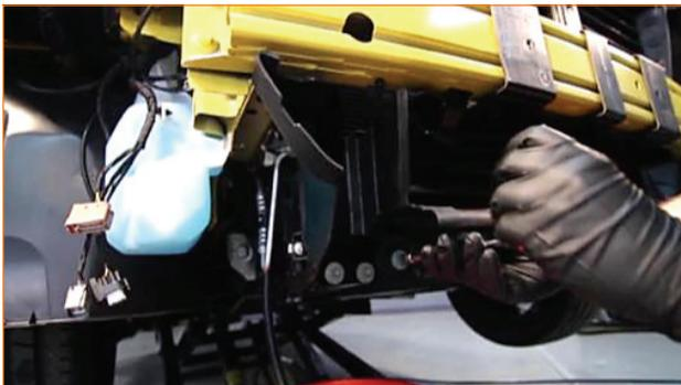
7. Separate the clip to free the air shutter arm.
