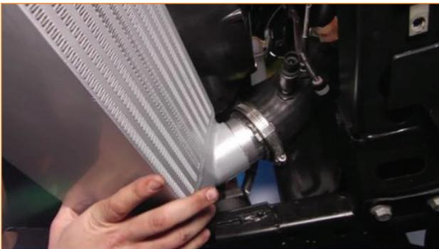
**26.** Tighten down the intercooler on the passenger side. (1x 10mm bolt)
