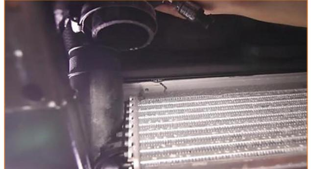
**16.** Remove the plastic cover from the side of the intercooler and rotate to the side.
