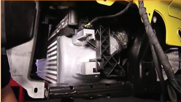
**33.** Put the plastic cover from the side of the intercooler back into place.
