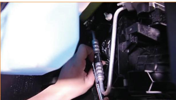
**15.** Detach the cold-side pipe from the intercooler.
