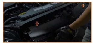
3. Disconnect the electrical harness at the back of the grille and remove the grille.
