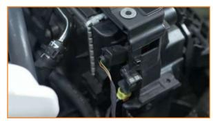
23. Separate the bumper support bracket that sits above the crash beam. (3x T30 torx bolts)
