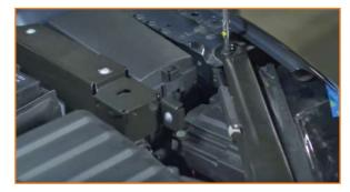
13. Free the hood latch cable from the support bar by compressing the gray tree clips that hold it. Next, separate the two pieces that hold the hood latch cable together.
