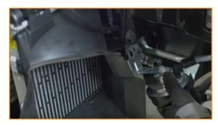
11. Disconnect the ambient temperature sensor behind the crash beam.
