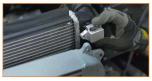
39. Secure the intercooler to the CNC brackets. (4x 10mm bolts)
