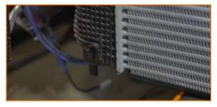
35. Release the tabs holding the intercooler to the radiator.
