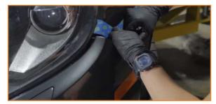
8. Remove the last two bolts securing the top of the bumper. (2x T25 torx)
