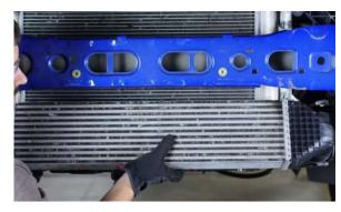
23. Remove the sensor from the end tank on the stock intercooler. (1x T25 torx screw)
