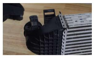
24. Install the sensor removed from the stock end tank onto the Mishimoto intercooler. Secure it with the bolt from your kit.
