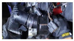
22. Tilt the bottom of the intercooler upward, and then lower it from the vehicle.
