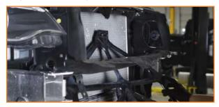
15. Disconnect the hot-side pipe from the intercooler end tank. (1x spring clamp)
