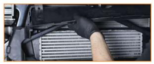
14. Remove the bolts that secure the bracket covering the intercooler. Two of the bolts can be found within the top edge of the engine bay. (6x T45 torx bolts)
