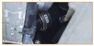
16. Disconnect the cold-side pipe from the intercooler end tank. (1x spring clamp)
