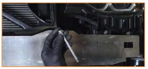
13. Release the tabs and clips to free the shrouding. Remove the shrouding from around the intercooler.
