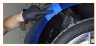
Disconnect the headlight washer line on both sides. Have a bucket ready to catch any residual fluid.
