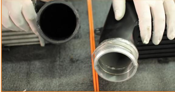
8. Lift the intercooler up into the engine bay and install it to the intercooler pipes. (2x retaining clips)
