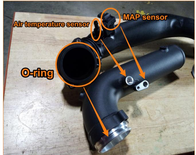
09. Swap the turbo side o-ring and the spring clip to MM2362-01.
