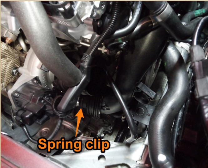
06. Remove the stock charge pipe from the throttle body.
