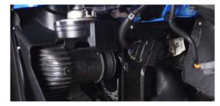
13. Loosen the clamp securing the cold-side hose to the intercooler end tank. Then, separate
