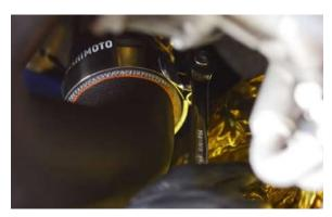
24. Slide clamps over the larger coupler and install one end to the hot-side pipe and the other to the Mishimoto intercooler.(1x worm gear clamp, 1x t-bolt clamp)
