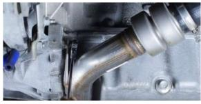
2. Loosen the clamp on the coupler between the hot-side pipe and turbo. (1x worm gear clamp)
