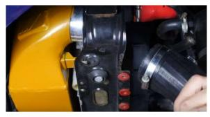
Slide a clamp over the shorter coupler in your kit and install it to the turbo. Leave the clamp loose for now. (1x worm gear clamp)
