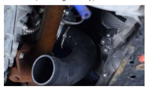
Install the intercooler pipe to the open end of the coupler you just installed to the turbo.(1x worm gear clamp)
