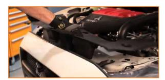
7. Unbolt the front bumper from the support bracket. (5x 10mm bolts)
