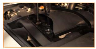
5. Remove the bolt that secures the airbox. Loosen the clamp where the intake hose meets the airbox. Then remove the airbox from the engine bay. (1x 10mm bolt, 1x 10mm clamp)
