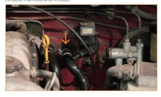
4. Using your 12mm socket, reattach the ground bolt to the engine block.
