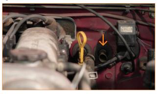
6. In order to remove the left heater hose from the vehicle, you must first remove the ground bolt from the engine using the 12mm socket. You will need to slightly bend the engine dipstick out of the way as well.
