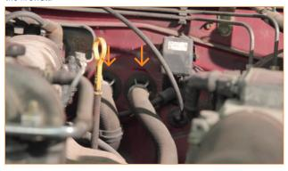
5. Working with care, carefully remove the factory heater hose on the right from the vehicle.
