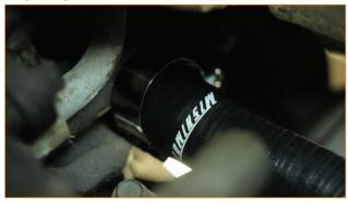
2. Reinstall the air box and OEM intake tubes by doing steps 2.1-2.3 in reverse. Make sure to securely tighten the 10mm bolts on the intake tubes, as well as the 12mm nuts on the air box.
