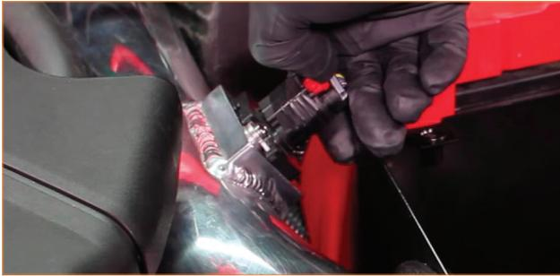
07. Remove the airbox isolator bushing. Remove the screw that runs through the center of the bushing. Then remove the bushing by pulling it upward. (1x T20 Torx screw)
