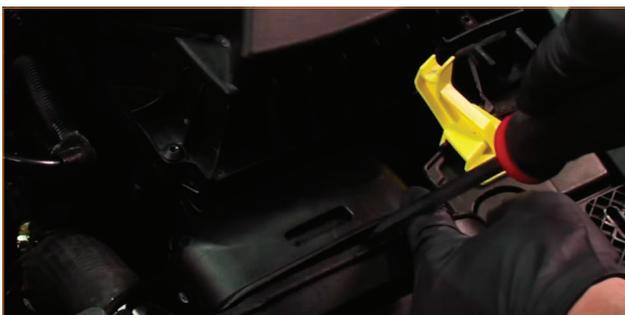
09. Locate the upper radiator hose. Disconnect the clip that secures the auxiliary coolant hose to the upper radiator hose.
