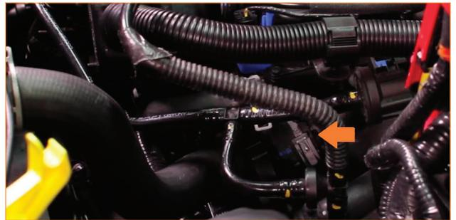
11. Using pliers or a hose-clamp tool, compress the tabs on the clamp that secures the upper radiator hose to the radiator, and slide the clamp down the hose. Remove the upper radiator hose from the radiator. (1x spring-clamp)
