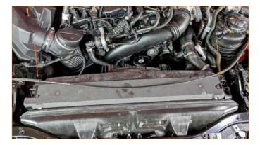
**31.** Reinstall the upper crossbar. Take special note of where the hood release lines go. (4x E14 bolts, 4x 13mm bolts, 4x 10mm bolts)
