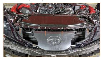
36. Reinstall the front bumper support. This is held in place with 2X T30 bolts (top) and 2X T30 plastic screws (bottom).
