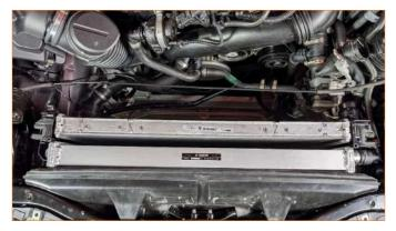
27. Reconnect the quick disconnects supply and returns on both the radiator and the heat exchanger. Ensure the locking ring is securely in place. Reattach the sensor's electrical connection on the back right side of the radiator. 28. Reinstall the lower radiator cover using the factory 2X T30 plastic screws. Again, take special care to ensure all plastic clips have been locked into place before doing up the screws.
