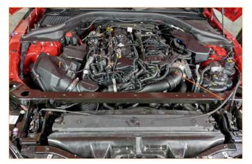
**32.** Reattach the transmission cooler. Slide tabs on the Mishimoto heat exchanger, then secure in place using 2.5mm allen tool. (2x M4X0.7 bolts)
