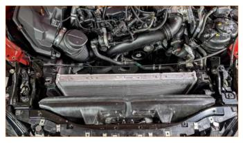
26. Next, slide the heat exchanger down from the top. This can be done without removing the radiator once all plastic pieces have been trimmed.
