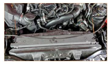
11. Remove the upper radiator cover. Simply unclip and pull off. (2x T30 plastic screws)
