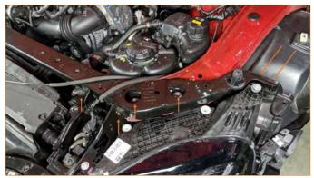
**10.** To remove the fan shroud, disconnect the electric plug on the back of the fan and remove plastic screws that secure it to the top of the radiator. (2x T30 screws)
