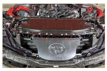
Remove the top metal radiator cover. Lift out of place once bolts are removed. (13x 13mm bolts)
