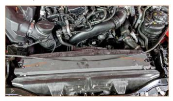
12. Remove the lower radiator cover in the same manner as the upper cover. Be careful where the inlet to the heat exchanger is you may need to use a pick tool to release a plastic tab up above the inlet.
