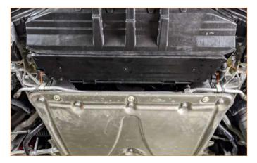
29. Install the top radiator cover. This needs to be placed in before the fan shroud since the fan locks into this. Use the factory T30 plastic screws to secure in place.
