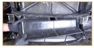
12. Remove the bolts that secure the cross brace and slide it out from behind the upper ducting. (6x T45 torx)
