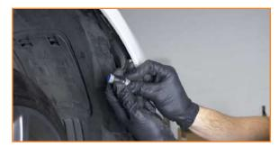
Disconnect the electrical harness within the wheel well.
